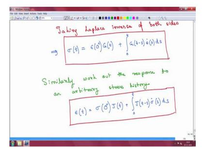
So, now, this implies that, so, now take Laplace inverse of both sides. So, let us just write that, so taking inverse of both sides you find that your on the left hand side you had sigma bar, so the Laplace inverse of that is simply is the sigma t or the function sigma t. Here, let us write this quantity first, so you have epsilon 0 plus the Laplace inverse of G bar is simply G t.
