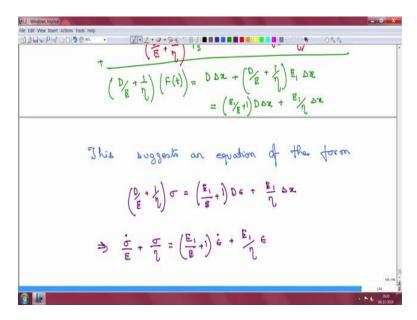
So, when it comes to the first is the Maxwell model or rather for the entire system, from geometry we can say. So, the geometry as we discussed earlier that is going to constrain the displacement, so that the displacement of the entire system is the same as the is going to be shared by the two individual systems.
