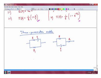
So, now what we can do is, but these were simplest possible models, which means that we can go on and build more and more complicated models. So, the obvious next step would be to build a three parameter model, we had only two. So, let us introduce one more complexity. So, there are different three parameter models that are possible.
