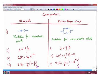
So, let us just do a quick recap, because we want to understand some of the key principles that are involved. So, let us just do a comparison. So, one side we have done the Maxwell model and the other one is Kelvin Meyer Voigt model, both of them are continuum models which means that we are using analogues disregarding the exact content atomistic basis for the viscoelastic system. So, we have not asked ourselves what is it at the atomic scale which makes this particular system viscoelastic.
