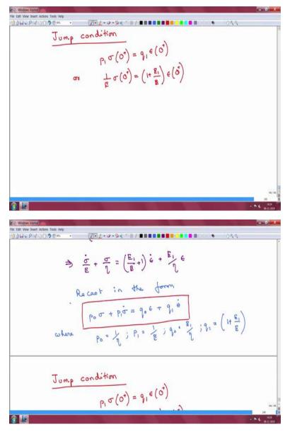
So, for both the Maxwell model and the Kelvin model, for the both the Maxwell model and the Kelvin model, we had discussed jump conditions and I had gone through details of how the jump conditions are to be found. In this particular case, I am not going to go through the same thing
