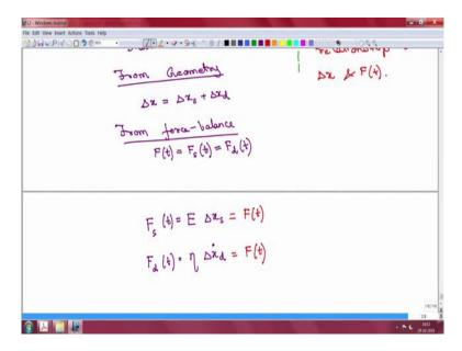
So, where we stopped last time was where we wrote down the equations. So we wrote down the geometric constraint equation how the delta X is and from the force balance we had written down the equation for the force, these are equal, this is rather straightforward equation. Then we had written down the separate relationships for F and this force in the spring and the force in the dashboard. So we will start off from here where we left off.
