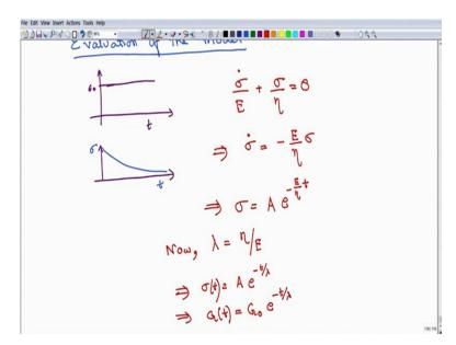
Now, if I want to write, now I introduce a quantity called lambda which is equal to eta times of E then the sigma is basically some constant times e to the power minus t by lambda. So, your GT so this is by the way a function of time maybe I will just make it explicit here and this implies that your stress relaxation function has a functional form of G naught into e to the power minus t by lambda and lambda here becomes a relaxation time scale. (Refer Slide Time: 08:15)
