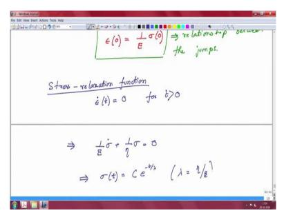
So, now that we have this let us go back to the derivation of the stress relaxation function. So we were looking at the stress relaxation, so our situation is that epsilon t is equal to 0 for t greater than 0 and our corresponding equation was 1 by E of sigma dot plus 1 by eta times of sigma equal to 0. So this sigma t is some constant times e to the power minus t by lambda where lambda was this eta by e.
