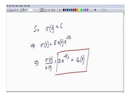
So, sigma 0 is equal to your constant and we know that sigma 0 is the relationship between the two is this. So this epsilon 0 is the given quantity is a quantity that we provided to you. So you can write it as sigma t equal to E times epsilon 0. So your stress relaxation function is actually this quantity. So this is your, so with the jump condition now you are able to get a proper equation for G.
