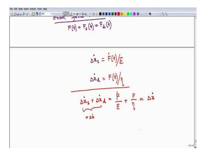
So now I am just going to remove this part because we have taken that out. So, if we take the derivative here and then we add up the two cases and we put this E on this other side. So let us say this E I am going to remove and I am going to put it in the denominator here and similarly I am going to remove eta on this side and I am going to take that here. Then you have your delta XS plus delta XD dot is equal to F. So I am going to not use this T because that is sort of understood.
