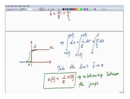
So, what we want to do the problem is being created by the fact that you are applying a discontinuous function. So instead of this discontinuous function, what we will do is, we will assume that there are certain continuous functions that are fully integral and this continuous functions go and merge into your original signal and there is a small gap of let us say plus minus delta.
