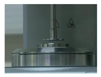
Once this calibration is done, the conal plate is taken back to another place at height of 60 millimetres.
