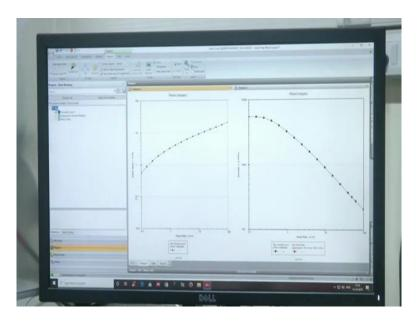
Moreover, in the rheometer, we also have the option to set the temperature conditions for the experiment. In this case, however we have set it to the room temperature. The data from the experiment can be observed in real time on the software screen in the form of an output graph. The graph on the left side shows the shear stress vs shear rate plot and the graph on the right shows the viscosity versus shear rate plot.
