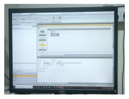
As you can see on the screen, the right side is the input. So currently we are setting the value of the strain to be 20 percent and we are collecting 100 data points.
