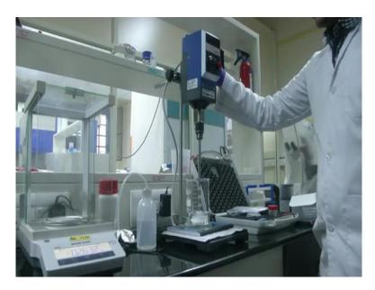
Next we fill the beaker with 100 ml. We then add the powder to the beaker. The PEO powder is available in the form of water soluble powder, which is how we will be preparing the solution today. Once we add the powder, we need to mix the solution properly to get a uniform solution.
