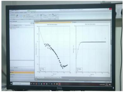
As you can see on the screen, the right side is the input strain and the left side is the variation in the fluid stress. The strain takes a finite amount of time to reach a steady value. So, while analysing the experimental data, we must be careful to remove the output stress in the region where the strain is not constant. Now, we have already done experiments for various other strain rates also. So, as you can see, the fluid stress is decreasing with time.
