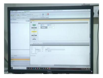
We now move on to the creep test. In a creep test, we give a constant stress input. In this case we will be giving a 100 Pascal and then observe the changes in the value of the strain. Similar to the previous cases, we first give the test name details. Then we set the value of the stress input and the number of data points.
