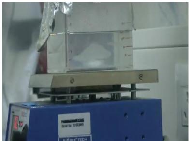
Next we move on to the magnetic stirrer. In the magnetic stirrer, we basically have a magnetic bead which is kept in the middle of the beaker which has the solution. Next we place it on the magnetic stirrer and set the RPM. In the current setup the RPM is set to 1000. It takes about 24 hours in the magnetic stirrer to prepare a uniform solution.
