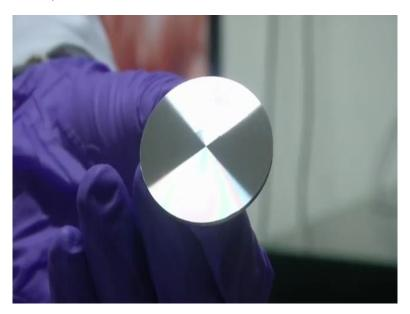
Now that we have the solutions prepared, let us move on to the experimental part of the demonstration. What you see is a conical plate, which has a 40 millimetre diameter and a 1 degree angle.
