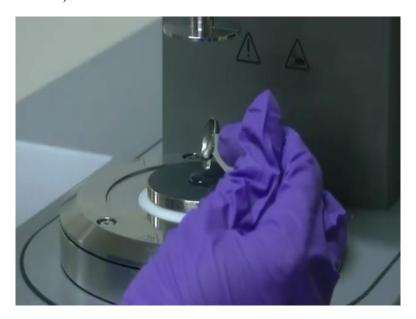
Once the plate is fully retracted, we place the sample fluid on the stationary plate. While placing the sample, we must be careful to place it roughly in the centre so that the conal plate can cover it completely.
