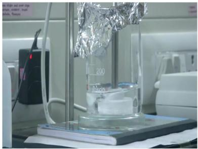
We will also be covering the top of the beaker using aluminium foil. This is done so to prevent any dust particles from falling into the solution. We will now set aside the mechanical stirrer.
