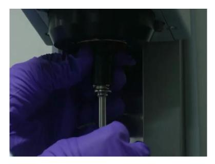
We then insert the rod into the measuring system. The conal plate has already been attached to the bottom of the rod.
