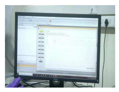
To run this experiment, we first open the required test module within the rheocompass software. This gives us the following user interface. We first enter the details of the experiment such as the sample name, the percentage concentration of PEO in the solution that we are using, etc. Next, we give our input commands. For the present experiment, it is the range of the shear rate.
