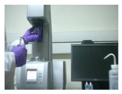
This is an Anton power rheometer with model number MCR 302. We will be performing today's experiments on this rheometer. So before we start our experiment, we will insert the conal plate into a cylindrical rod and then attach the cylindrical rod to the measuring system. Before we do that we need to remove the protective covering for the measuring system.
