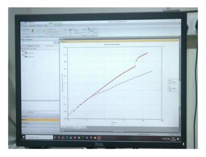
So, you can see the changes in the value of the strain for the given stress. That is you see the creep compliance varying with respect to time. In the creep experiment, it is the variation of the creep compliance that is of interest to us. For this test, we have also performed the experiment under stress of 200 Pascals.
