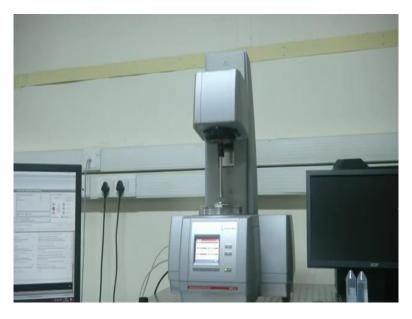
In the first part of the calibration check, the software tests the motors of the rheometer to ensure that it works properly. After this, it goes for the zero gap check. In the zero gap check the conal plate geometry is brought very close to the lower stationary plate. The actual value of the zero gap is pre-set.
