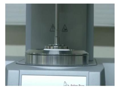
After the plate is lowered completely, make sure that it subsumes the fluid. If there is still some excess fluid around the outer edge, then it must be trimmed off before we start the experiment. Now we can start the actual experiment. We first begin with the flow curve. The flow curve measures the viscosity of the sample with respect to the shear rate.
