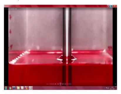
So going back to the rod climbing effect, we as I said, two people from my lab, they did an experiment, Navin and Udita and what you have here is this a rod that is partially immersed, this is a rectangular beaker and you have a polymeric fluid here. So you have a polymeric fluid that is there in the system and this is a rod and we are going to rotate this rod at a particular angular velocity.
