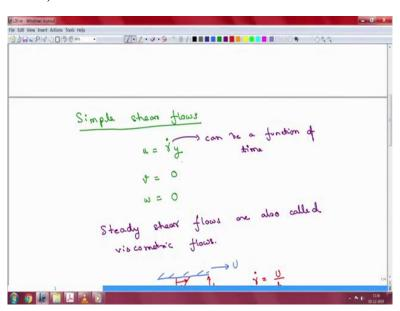
And here we had said that the function u is function of y and is given by the flow field is given by these velocity fields where we have written it down in the competent forms so we have U, V and W as the velocity components.
