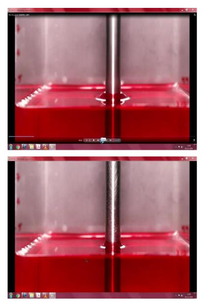
So let us quickly look back at it one more time. What we saw. So this is a fluid at rest, you have the stationary meniscus, which is formed right around the rod and you can see the difference. So you can see clearly this very large rise. So this is the rod climbing effect.
