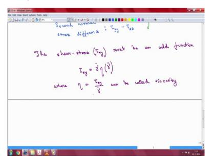
Now, this shear stress here, so this shear stress must be an odd function. I mean you can look at the, you can probably figure that out from the physical argument that is the direction of flow changes, then Tao xy sign should change. Its value is the flow remains exactly the same, but the direction of u is reversed, then Tao xy will have the same value but with a different sign.
