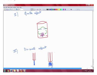
There is another related effect, which is called the Quelle effect and in this system, what you can have is, let us say you have a beaker and instead of rod that is partially immersed, you have let us say, an impeller here inside that is fully submerged and you have fluid in this. Then when you start rotating it, what can happen is you can start to have a bulge here because of secondary flows that can occur in this region.
