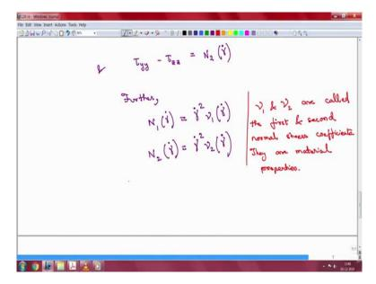
We can also argue and show that the first normal stress difference Tao xx minus Tao yy and, and I am just going to complete this in a second and the other one which is the second normal stress difference, they are actually even functions. And you can write this as some N1, which is an unknown function and it is dependent on gamma dot.
