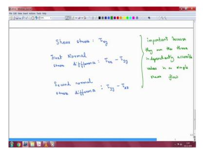
Now, they are important because they are the three independently accessible values in a simple shear flow, so important because they are the three independently accessible values in a simple shear flow, experimentally accessible.
