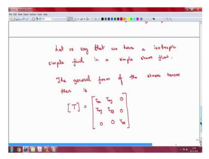
So now, let us say that we have a isotropic simple fluid in a simple shear flow. We know the form of the velocity field but the question is what is going to be the form of the stress tensor? So we want to now understand how the stresses in the fluid are going to develop. Now the general form, so to say the general form of the stress tensor then is, so let us say we have a stress tensor, I am just going to write it in matrix form.
