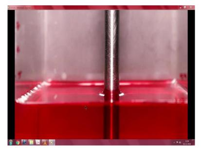
The rod is stationary now and it is going to rotate. So I hope you saw how this meniscus rose here. So this is called the rod climbing effect. If you go to higher polymer concentrations and higher rpms, this effect can become even more drastic. Here I believe the omega is something, so the rod is being rotated at around 1000 rpm and once the rod stops moving, the fluid just goes back to its original rest state.
