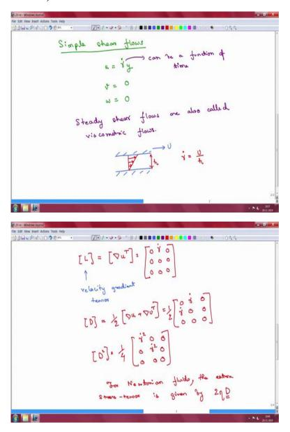
So, let us look at simple shear flow is such flow, where the velocity field is given by, so you will have three components of velocity for any given general flow. So, for a simple shear flow, we say that the velocity should be of the form you should be have some gamma dot times of y, we will clarify why we are writing it as gamma dot is basically some constant times y.
