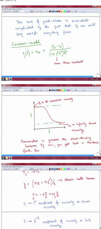
So, and in a Carreau model, the equation that governs this is given as, I am just quickly check what was the term I was using for, so we have been using eta for viscosity. So, maybe we will just stick with that. So, eta gamma dot, so the viscosity when we wrote this in it in this way, it implies that your viscosity is a function of the shear stress is usually it denotes one constant, which is eta to the subscript infinity.
