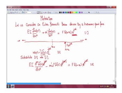
Since I work in the area of vibration and acoustics, I will take the example from vibrations. So, let us consider an Euler Bernoulli Beam. Those of you have had a course in vibrations would know this. This beam is now driven or excited by a harmonic point force. So, the equation of motion can be written as EI del 4 w del x 4 plus m dash del 2 w del t square and there is a point force applied at x equal to x 0. It is harmonic, so we have the time dependence and this is an infinite beam.
