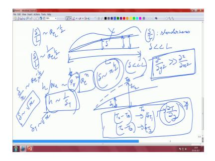
So, if I try to plot this particular thing that not plot, but basically see the dependence right Reynolds number to the power of minus half. So, that is the relationship that we have initially right. So, this as I say, it is nothing but the slenderness ratio so; that means, if this is the boundary layer that is growing right, this is delta this is L right L or x right...
