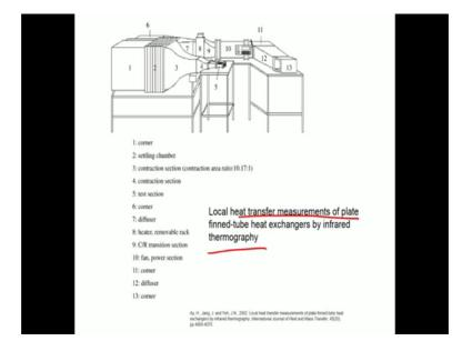
Now, other examples this is from our group there could be other examples like for example, this is a wind tunnel experiment. You want to measure the local heat, transfer between a plate, finned heat exchanger using infrared thermography that is one other kind of measurement that you might want to measure ok.
