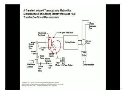
So, another thing could be a transient thermography measurement technique for simultaneous film cooling. Film cooling is what we use in the gas turbine plates right. So, for film cooling one uses this infrared camera and that the film cooling setup is right here and you can use it in a wind tunnel and you can measure what is the temperature ok.
