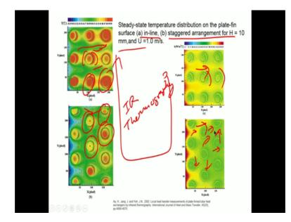
This is for example, in the steady state temperature distribution on the plate fin surface. So, you can see the temperatures right all these places these are temperatures you can see the linking between the two which is happening because of the flow right. So, there is a fore and aft asymmetry of the temperatures correct you can see the wake patterns very clearly right, but how each of these holes are dominating each other correct is not that so ok.
