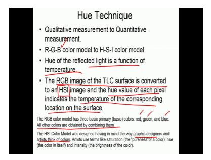
So, the qualitative measurement to quantitative measurement what we want to do is basically you want to go from a R-G-B type of model; R-G-B is the red, green and the
