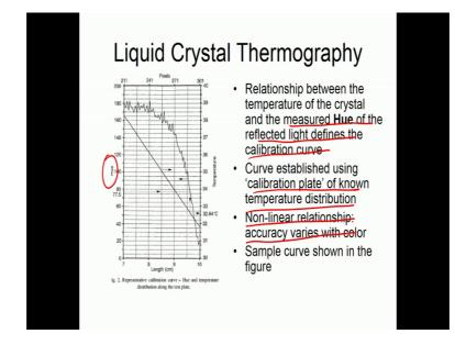
So, the relationship between the colour and the and the and between the temperature of the crystal and the measured hue of the reflected light defines the calibration curve, ok. So, this is the hue, ok. The colour established using calibration plate of known temperature distribution, as I said is a non-linear relationship accuracy varies with colour, and this is one of the sample curves that we have shown, ok.
