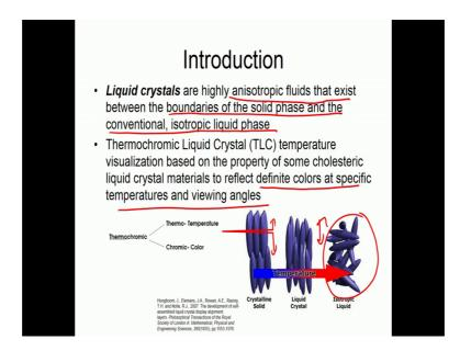
So, if you look at the slides now, you will find that what are liquid crystals? Now, liquid crystals is something that you already know, right. Liquid crystals you see it for example, in LCD TV's are usually made out of liquid crystals, right. So, liquid crystals are basically highly anisotropic fluids that exist between the boundaries of the solid phase and conventional isotropic liquid phase. It is neither solid nor liquid it resides somewhere in that boundary, right.
