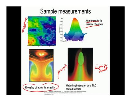
So, these are more sample data say for example, this is a surface where TLC, TLC sheets have been pasted and you can see the temperature distribution, you can see all the temperatures ok, marked out. So, with very good resolution you have been able to get. This is heat transfer in narrow channels ok; this is for example, water impinging on a TLC coated surface this is freezing of water in a cavity.
