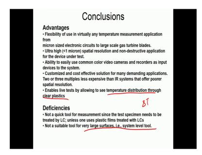
So, advantage is that flexibility of use in virtually any temperature measurement, and it has got ultra high less than a micron order spatial resolution, non destructive in nature, you can use common colour cameras; that means, DSLR cameras and other things can be useful and it is a low cost things, low cost than any other system that we can do ok, enable life test, but you can see the temperature distribution also, right.
