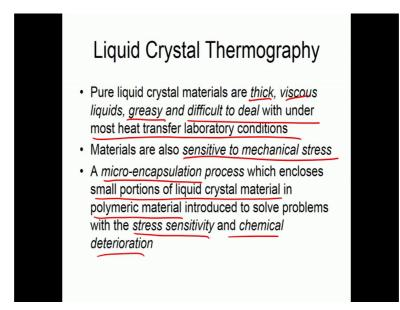
So, pure liquid crystal materials are thick, viscous, greasy and it is very difficult to deal with under most heat transfer conditions, ok. See these materials are also sensitive to mechanical stress, right. So, micro encapsulation is a procedure by which it encloses the small portions of the liquid crystal material in a polymeric polymeric polymeric shell ok, through it actually solves the problem of stress sensitivity and chemical deterioration, ok.
