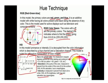
So, the RGB or the red, green, blue in this model the primary colors are red, green and blue it is an additive model; that means all other colors are basically added. So, in the RGB colour space if you look at that say for example, the colour with a P are the primary
