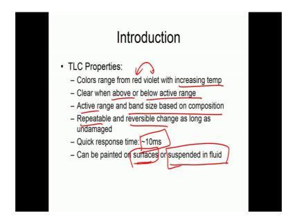
So, the TLC's the colour changes from red to violet with increasing temperature, some of the properties clear when it is above and below a certain active range. So, these TLC's has got active ranges. So, if your temperature is too high it will blank out, if your temperature is too low it will blank out.
