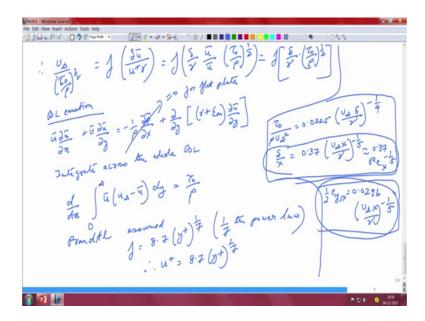
So, therefore your u infinity by tau naught by rho to the power of half because u bar is equal to u infinity at the edge of the boundary layer that is nothing but a function of delta u bar divided by u plus by gamma or in other words this is f delta by gamma.
