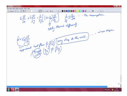
And we will pick it up start it here we will pick it up in the next class. So, this is the total equation once again we have assumed that d by dy is greater than d by dx is the boundary layer assumption. So, this exactly looks like a like your laminar boundary layer except that you now have this eddy thermal diffusivity coming into the picture.
