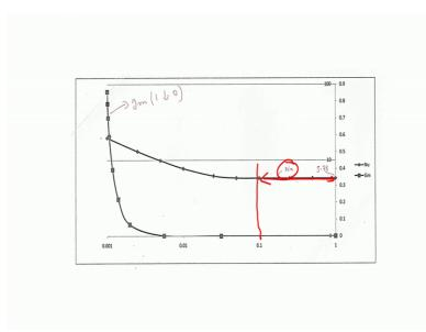
We can show that this is how the entire thing actually works. As you can see the, this is a mixed mean temperature and this is the corresponding value of nusselt number. Once again it starts off pretty high at around X bar is equal to 0.1. It slowly asymptotes to the value of about 5.7831 and after; that it is constant. Because that is the thermally developed regime and the only thing is that here u is equal to capital U. So, that is the only caveat that we have in this particular case.
