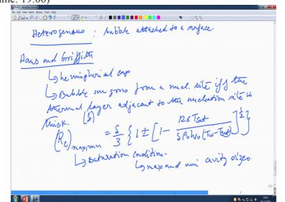
Now, in the case of heterogeneous bubble growth, heterogeneous bubble growth, okay. So, this is attached with a surface, right. Bubble attached to surface, okay. Now, the vapour bubbles attached to a heated surface basically, the growth occurs in a non uniform temperature field, okay to say the list, okay.
