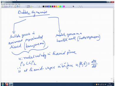
Now, let us now look at the Bubble dynamics. Now, in the case of a Bubble dynamics, what happens is that there are two types of Bubble dynamics that you can see, when the bubble grows, when the bubble grows in quiescent, superheated liquid, it is basically homogeneous, if you recall what is homogeneous and what is heterogeneous.
