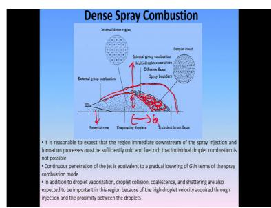
There are in the case of jet flame, you have a little bit more suggestive thing. For example, there is an external group combustion behaviour, as you can see. So, this is the group combustion, okay. So, there are multiple flames present. So, this is for example, the individual droplet clouds.
