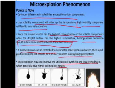
So, Microexplosion happens. So, there has to be an optimum difference. The low volatility component will drive up the temperature. The high volatility component will lead to internal nucleation. So, both the components have got their own role to play, okay. So, the droplet Center has got the highest concentration of the volatile component while the droplet surface is the highest temperature.
