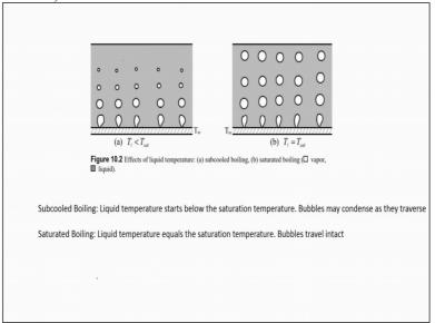
So, we will there are different types of boiling and there are different types of other things which we are going to do in the in the following lecture where we are going to see that boiling is bubbles essentially, the story of bubbles like we had the story of droplets, it is the story of bubbles. This boiling can be of different types homogeneous, heterogeneous, nucleate, there are different core classes of boiling, okay.
