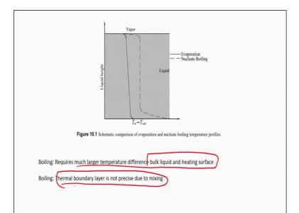
If you look at this particular little slide over here, boiling is not evaporation okay; once again, we are going back to Amir Faghri and Yuwen Zhang book, okay. So, boiling requires much larger temperature between the bulk liquid and the heating surface than evaporation, right. So, you can have evaporation and you can have boiling as you can literally see, if the evaporation curve is this.
