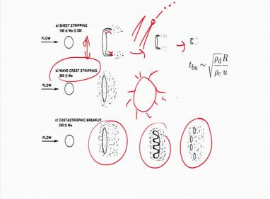
So, just to finish before we finish this particular part of the lecture, we see that vibrational mode of breakup happens like this. So, there is a nice spherical droplet, it just deforms like this. It is a single mode and then it used to generate two dotters. And this might undergo this cascade once again okay.
