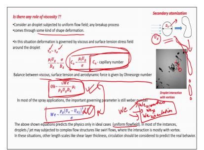
So, what is role of viscosity now we have said that it is inertial by surface tension, right, essential, right. We have not said anything about the viscous force at all. Now you know that the break-up process is not an instantaneous process right. So, you have a droplet which is facing this gas phase flow field right that is what we covered.
