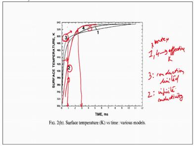
So, let us look at the surface temperature on the other hand based on the different types of models that we have over here okay. Now if you look at the surface temperature once again 1 and 4. You should recall 1 and 4, 1 is a vortex on the extended model okay, 4 is the effective conductivity model, K model.
