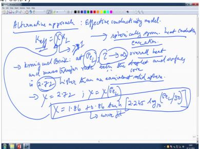
Now there is one more alternative approach, I am sorry, so, there is one more alternative approach and this approach is basically called the effective conductivity model and what does it do essentially okay. So, what it does is that instead of using the actual conductivity, the thermal conductivity.
