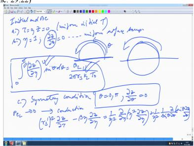
So, this has this is subjected to some initial and boundary conditions a. Tau = 0 t = 0 this is the uniform initial temperature right as the initial temperature, b. at Nita = 1 that means at the surface of the droplet dz by d theta = 0 okay this is also again uniform surface temperature at any point. If we said right the surface temperature is always uniform regardless right, okay.
