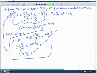
So, the phase change happens very fast, okay. So, we can assume that equilibrium conditions prevail, got it. Since equilibrium conditions prevail, we can write the Clausius-Clapeyron equation okay to link the mass flux to the YF basically. The species mass fraction to the corresponding temperature at the interface, right.
