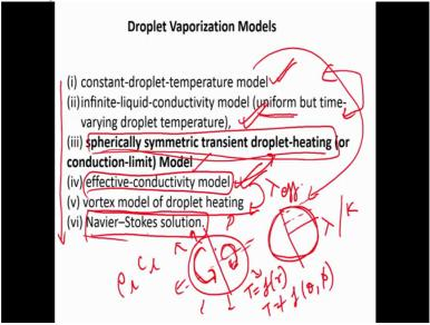
Like the different droplet vaporization models and we are going to go one by one, okay. So, if you look at the first simplest model is a constant droplet temperature model, right. Now, this is the model that is going to yield you the d square law essentially, okay. There can be also infinite liquid conductivity model it means that the liquid conductivity, the liquid temperature.
