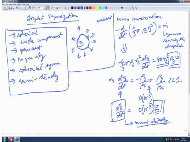
So, Droplet Vaporization, okay. So, as we know, if you recall the previous lecture, it is a spherical droplet vertical in shape; single component. Let us not assume multi-component
