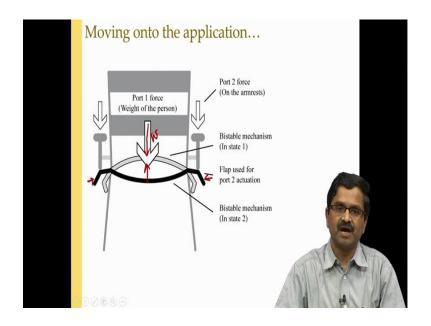
We have the bistable that his up that the weight of the person comes we go to the black one so that is the bistable and then the handles when you do that is port 2 actuation that is a actuation like this it will again switch back to that one, but then the continuously this weight is going to act so for that we have this static balancing.
