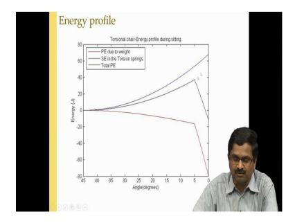
So, that is how energy profile is going to look like it is always is going to apply force here. We are showing total potential energy standard energy in a torsion springs and this, it is going to keep on increasing the total p that we have.
