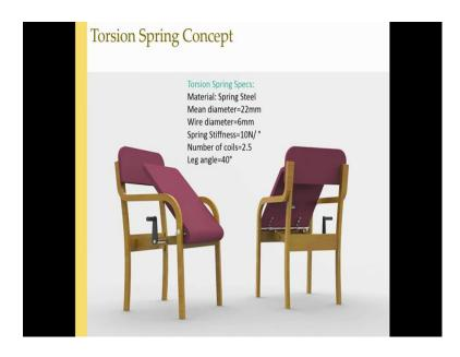
So, if you put a simple torsion spring here this is the prototype there is the simple torsion spring over here when you sit on it; it just comes down, but it will always be applying force on you that is the drawback of this simple chair.
