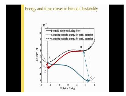
It has one path to go from one state to other state and a different path to come back - blue path while going the red path will coming back. Red path requires much less force than blue path and because the energy is stored in this bistable device. So that is the bimodal bistability and we have discussed all of this in a previous lecture we can pass the slides and look at a there is optimization problem that was solved and all that is analytical 1.
