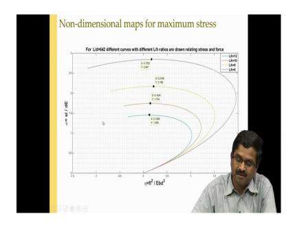
And looked at with maximum stress because we do not want to design a spring that is going to break because elderly arthritic already weak people, we do not want any catastrophic failure any product we looked at the maximum stress also and design some prototypes.
