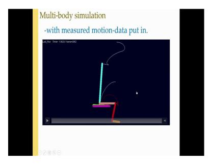
And we also looked at multi body simulation with a measured motion of the data of the person and you can see how their head goes forward when they are sitting with a particular motion and sit there. So, that is how we sit, when we are sitting it bend forwards a little bit and then come here. We can do this for each person based on their anthropomorphic proportions and their weight and so forth.
