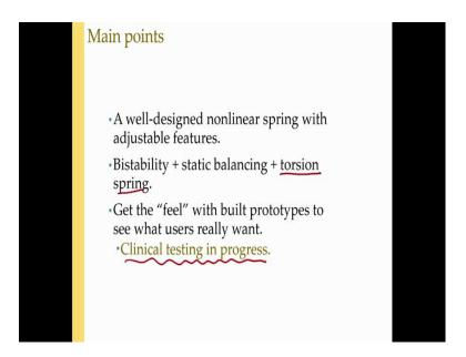
The main points here - we have a well-designed non-linear spring with adjustable features that combined by stability and static balancing and also if one wants a torsion spring because it is simple to do, it is should get the right feel by the users. Right now we are using this chair in nearby a hospital with Doctor Medha Rao with geriatrician who is with all human ethic clearance is testing it in the clinic to see it what the patients say -
