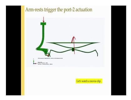
This is what it shows, if this is the seat where you can put a cushion it comes down person sits and then the handle when the force is applied here it would move here and it will switch back so that is the idea. So, bistable bimodal; so, it is 1 stable state, it can be other stable state.
