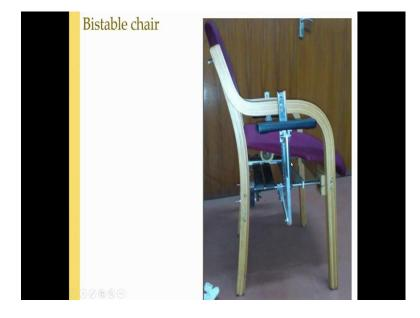
So, this is the prototype and this is the one where there is the handle also which will gently go. So, we have static balancing and this combined will get you this. Putting it all together this is the bistable one static balancing lot of mechanical details, now trying to get it all with much simpler design, but still having the same concept of bistability combined with static balancing.
