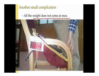
So, this small complication is that the weight does not come all at once when you are sitting. So, the chair is here like this when the person sits entire weight of the person does not come. So, we have to do static balancing for variable load here. So, we did some studies on how the weight comes by putting a load cell that is shown here.
