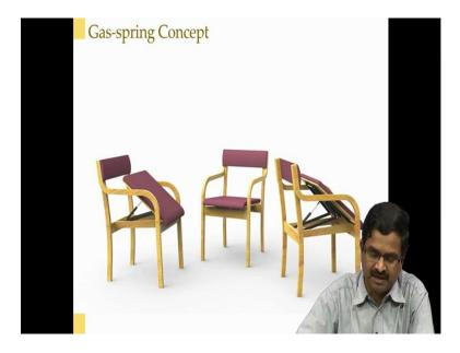
Slider crank - gas spring type of thing which is slightly better. So, this also has a gas spring different weights we can put different springs here so that when person sits according to the weight of the person we provide some assistance since this slider crank has some nonlinearity here there is a little bit. So, while sit there is not that much of a force trying to push you, but it is not 0 forces like in bistable mechanisms.
