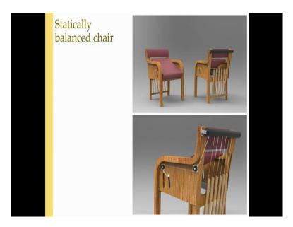
So, we had put this springs at the back of the chair, so that it actually becomes floating that is with the weight everywhere it is perfectly balanced that is what we want to, we want to composite on the weight of the person when we couple it with the bistable mechanism.
