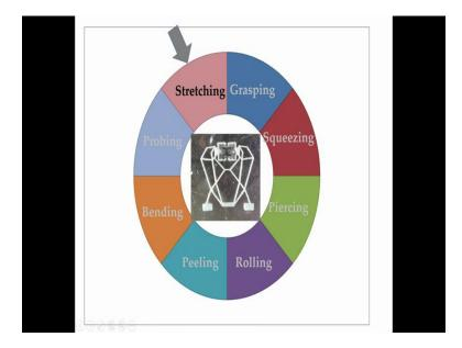
And stretching we had already seen. One point to notice here is that the material of this mechanism under one insight they are different. So, the reason is that if you use lithography and make the micro compliant mechanism here it is suppose to grasp something and then stretch you need to have very tiny beams. So, those tiny beams
