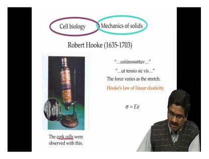
So, always start with this microscope image. To say that it was Robert Hooke, one of the pioneers in two fields cell biology and mechanics of solids because the Hooke's law that we talk about today is credited to Robert Hooke who said using an anagram in Latin "ut tension sic vis" which means the force varies as the stretch that is what he had observed.
