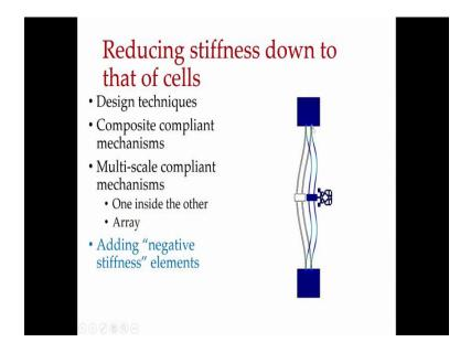
Negative stiffness is we have talked about bistable elements. Bistable elements over a small range they have negative stiffness. If we attach that preloaded along with the gripper then the gripper overall has some positive stiffness. This has negative stiffness over a small range you put them in parallel overall the stiffness would reduce; that is the idea we will reduce by even order of magnitude, so to get down to that level.
