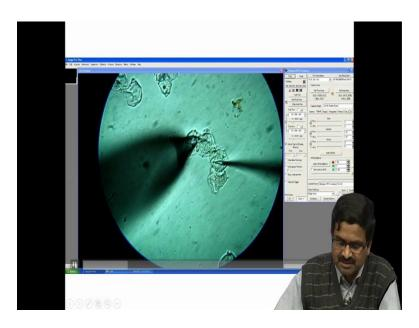
So, it is more of manipulation capability with the probes and the probes are attached to a compliant mechanism that measures forces. We can peel one cell which attached another one by just tearing them a part.
