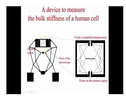
Accordingly you can design and putting one inside the other we already talked about where you have one mechanism that gives the parallel jaw motion and within that we put two DACM's. And this is where the cell is going to go. So, this tiny space is where the cell is going to go these beams are only 5 microns wide. And the cell as we can see that is also a few microns.
