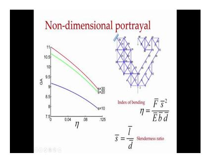
And we also use these non-dimensional maps to understand the capability of geometric advantage, mechanical advantage and the force requires stresses and so forth in doing this.
