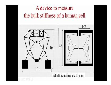
And this 1 is 10 millimeters by 10 millimeters, this big mechanism. Within that there is only 1.7 by about 1.7 so about 2 millimeters thing and these things are very small. They
