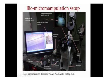
This is a set up in our laboratory. This is a digital microscope that measures the output displacement and gives us the force, while compliant mechanisms are actually manipulating the biological cell
