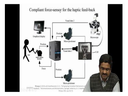
With all of these things force sensing can also be done compliant mechanism; not only manipulation but also force sensing which we will discuss in another lecture. But what we will focus on here, in fact this is the force sensor compliant mechanism. There is a
