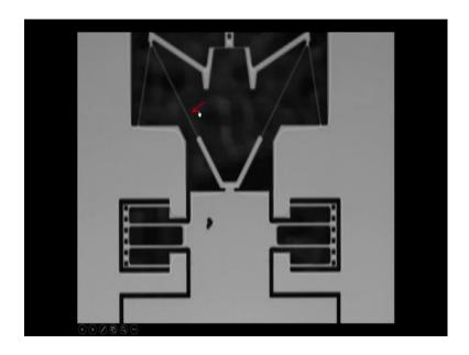
And there is a close up view we will see the movie. So, you can see these things they are so thin they are more like you know wires or strings, but it is silicon and it does not break; we have used it packaged it and all that it works in most of the beams in micro electro mechanical systems devices are really thin, and they work and you do not have to worry about the breaking.
