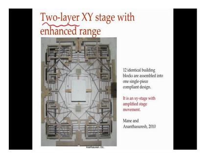
Now, here is one that was made with wire EDM, looks complicated. It was aluminum or spring steel very complicated device lots and lots of beams and its was made in two layers - it is an xy-stage with enhanced range. So, metals also can be used very happily.
