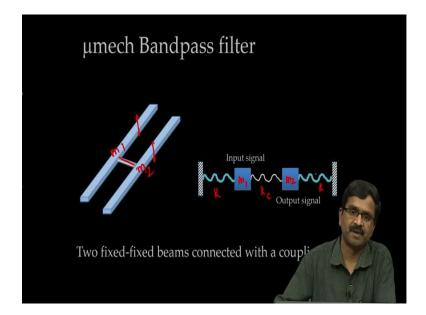
In order to look at that as a model let see that this is 1 beam that moves up and down another beam that moves up and down and this is the coupling beam how do you represent it? It is like this; the mass of this, so there is this mass m 2 and m 1. So, we have m 1 and m 2 of course, these things are now shown to move in plane, but it could also be out of plane.
