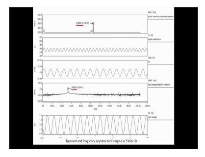
And here is another example where input is a 53000, output is 106000, frequency doubler this one is.
