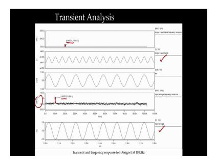
The input is here and output capacitance is here, where the frequency is doubled for the signal and in fact, if you do the db the frequency response you can see that this input is in this case 1 lakh and the output is 2 lakhs there is a peak there everything else is, you know frequency response is very small, db scale it is very large db to 300 to 50 and here is 100. So, we can see that we can use a little compliant suspension to do the frequency translation.
