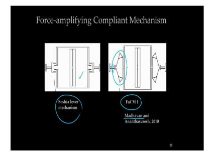
Again coming with suspensions is important here as was done this was one mechanical literature what Shyamsananth Madhavan had done using FaCMs that is force amplifying compliant mechanisms. We have a few mechanisms of that kind also these are force amplifying mechanisms there were design using optimization where you can have the natural frequency in the beams that are here and lot more change for the same
