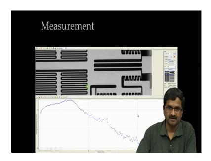
We measured it and it actually works like a the frequency doubler and then move it on to frequency quadrupling also that is f comes and for f goes out as output.
