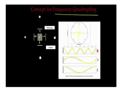
Here what we need to do is we have to have a mass actually move symmetrically with respect to 4 electrodes in a fashion like this, it moves this way that way combination, if we do it this what is shown as a clock 1, 2, 3, up to 8 as the mass moves you have symmetry and all four sides. So, input that is a wide movement at one frequency, x
