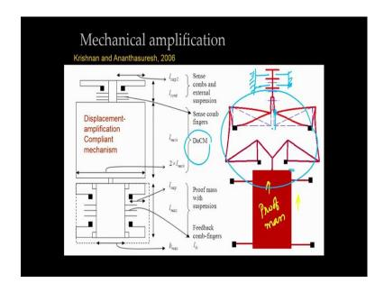
Here is a an accelerometer where we have the proof mass, this is the proof mass then there is acceleration which going to move, if I measure the displacement of this mass here that is not going to be very much instead if we measure someplace else if we measure someplace else meaning over here see how much it as moved so much and you can hardly see any displacement of this.
