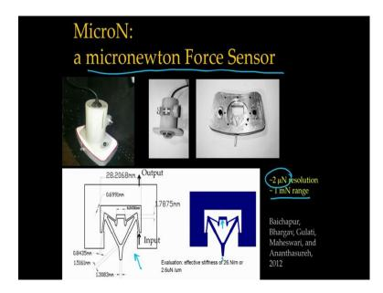
Now let us look at a micronewton force sensor that also uses a compliant mechanism that is shown over here, we may apply some force this is going to move a lot more and give you in 1 millinewton range the resolution about 2 micronewtons.
