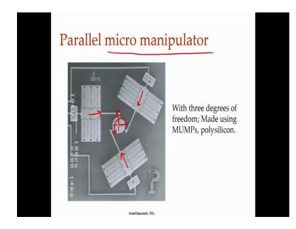
And one can make a parallel micro manipulator which has three degrees of freedom; x motion y motion and rotation by changing voltage here and these are like parallel (Refer Time: 22:08) that will expand and contract and you can actually make it like a parallel planar parallel manipulator.
