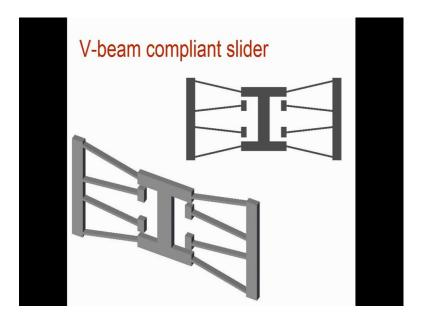
Here is a folded beam suspension and, but that is for ortho planar motion; that is some that lifts out of the plane with certain stiffness characteristic. Here is a variant of the folded beam suspension where there are V-beams instead of parallel beams and this is a very interesting two axis micro mirror mechanism, which was done by a gear which was spin off from 8 into bell labs and bell labs was closed down.
