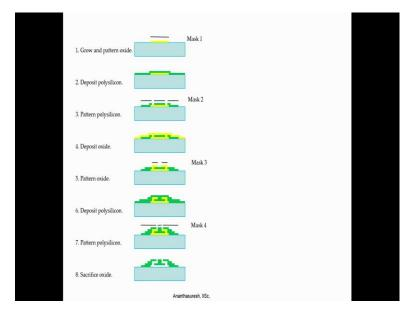
So, process for that is re-elaborate; you need four lithographic masks so make it, instead what people very quickly in the MEMS field realize is that; instead of making a slider that can go in and out now as we showed in the previous slide that can slide like this. Instead of that one can go for a compliant slider.
