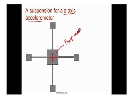
So, very popular suspension mechanism with basically replicates the prismatic joint without having to have rubbing surfaces or assembly or where or friction. A suspension for a z axis accelerometer because this one will be very stiff in the in plane directions, but flexible in the out of plane direction so that becomes is z axis accelerometer, where
