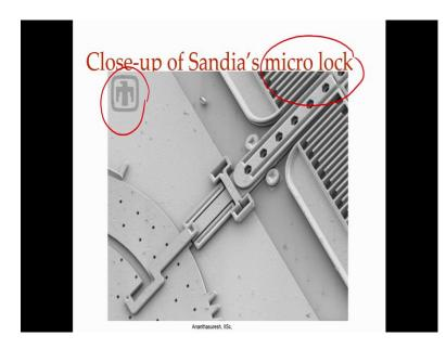
So, all of this required sophisticated micro fabrication process, and here is a zoomed in view of the gears and slider and pings and so forth that came from Sandia national labs.
