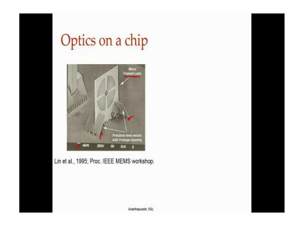
But or they could make optics on a chip here is a Fresnel lens that is actually made to stand upright on a chip and this little thing here is says this is 40 micron. So, this little bar over there we see a little bar was 40 micron second, you can see how small it is. Gradually there are some locks here and there all done on the chips so that what is made flat to be planar is actually pushed up to become 90 degrees or perpendicular to the chip.
