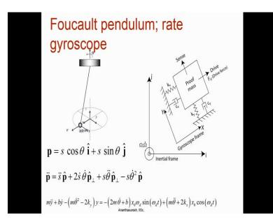
So, you can look at that, so you can have a pendulum suspended can have motion like this or motion like this in a perpendicular way. So, you put energy into this when the frame starts rotating then it will change the plane.
