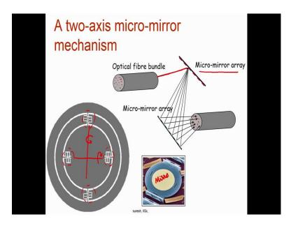
What we have here is a mirror which is shown here, it can tilt about this axis; it can also tilt about that axis. So, it can tilt like this and like that which is used for optical fibre
