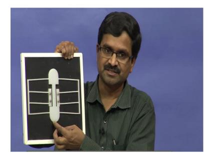
So, here is the folded beam suspension, so it is fixed over here and here and very easily there is not that much stiffness here and if I start moving it here its actually quite difficult I cannot actually move in the x direction it very stiff I can I cannot move it.
