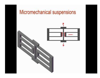
And there are number of suspensions, this is a folded beam suspension which is fixed over here and this one will be very flexible with that direction this direction, but very stiff in these direction.
