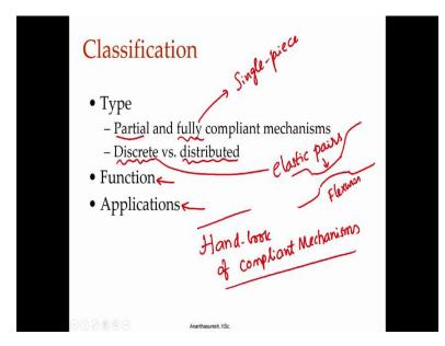
So we think about classification of compliant mechanisms; one can do it in various ways, first is type. We can say there are some partial compliant mechanisms where all members
