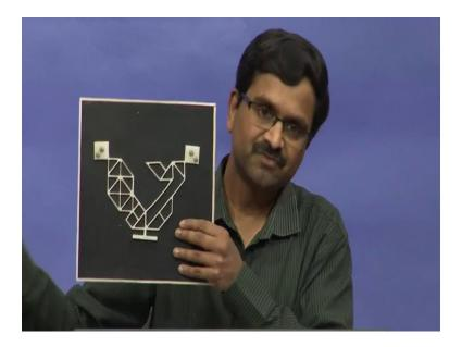
And here is one that was the basis for designing what I just showed. This was algorithmically designed, so here amplification is there by about a factor of 7, but not as much as the other one. So, that was inspired by looking at this; this was designed using topology that mention algorithm by Anupam Saxena; who is now a professor at IIT Kanpur, but this itself has inspired several applications for us.
