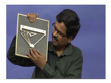
Here is one - this is the top portion is completely fixed, there are screws and then all made with polypropylene, these just the material we used to make this model, but because of our Kineto-Elastic maps the same design can be done with any material, any size, any cross section; as we will also discuss later about what materials could be use for compliant mechanisms and what manufacturing techniques will be used to make compliant mechanisms.
