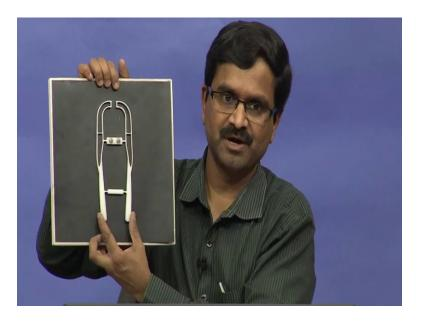
This is a parallel motion gripper when I apply equal forces at these two points and these two things will go almost parallelly without rotating. By that I mean they go like this; not like an arch motion or going like this, they can actually go like this without this tilting or this motion, they just go like this.
