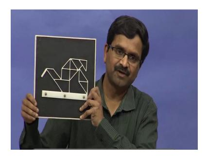
So, let me start with one over here, but direction changing what I am mean is that apply force in one direction and the displacement will be some other direction. This one was designed using an optimization algorithm again by Anupam Saxena, who is at IIT Kanpur now; he is professor there. So, apply a force in the vertical direction I am pushing it down, see where the output goes, it goes in that direction.
