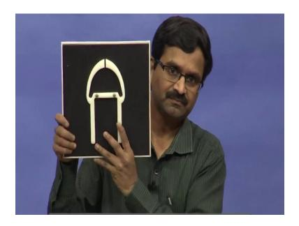
Now, let us move on to clamps, so clamps are there everywhere. So here is one, where I press like this; it opens up, you put some object over here and then remove it; it holds basically even the board is held by just my hand now because it is gripped. So, it has such a good clamping force; so this is like a clamp and that can be used.
