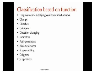
What we have today are classified compliant mechanisms or compliant mechanisms classified based on functions, we look at examples of each of these.
