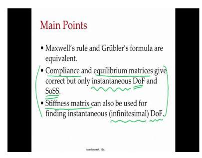
We have a few points to note that Maxwell's rule and Grubler's formula are equivalent when one fails the other one also fails, both work by counting in the case of Maxwell's rules number of rule number of vertices the number of bars Grubler's formula number of bodies which is number of bars, but also the joints and the type of joints and so forth.
