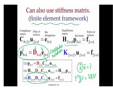
And we can also use stiffness matrix which is from the finite element framework here we have the compliance matrix relating displacements and bar elongations equal to the matrix relating bar forces and forces acting on the vertical external force, but what we want is actually the stiffness matrix.
