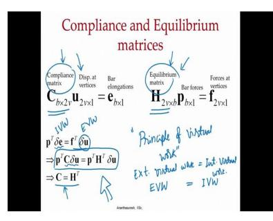
And interestingly these two matrices the C matrix and H matrix the compliance equation matrix equal equilibrium matrix have a relationship that is shown here which follows from the principle of virtual work.
