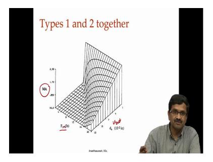
And you can look at both of them together as well type 1 type 2 3 parameters you have F in and then u out there you they use d o it is from their paper mechanical advantage both type 1 type 2 you can imagine like a surface the slices of this, that is fixing F out you will
