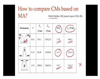
And if you do this for different mechanisms as Mohit had done you can see that a mechanism that has high MA s has some sensitivity, if I go to other mechanism that has let us say low MA s also high sensitivity this actually very bad anyway, it is a gripper does not have mechanical advantage where as these are the one that can actually crush things over here the output this the output here this is input.
