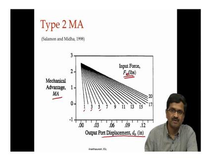
Let us look at type 2, in type 2 for different forces. So, you fix the input force. So, input force are 1 2 3 5 whatever we get different ones here, now output displacement is there not output force output displacement varying and then you have mechanical advantage.
