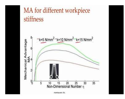
So, you can look at (Refer Time: 31:14) work piece stiffener, let say how does mechanical advantage change with respect to work piece stiffness.
