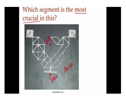
Let us say we have the same mechanism n apply a force, which going to blue like this with a lot of output displace which a Displacement amplification complain mechanism, these what was given by topology optimization lot of beam segments are there, which of them is the most crucial, if you ask the question, what we could do? When you draw the maps is draw all of them.
