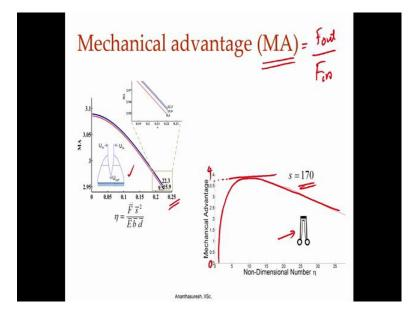
So, there are things like that you can store for a mechanism, we can also do with mechanical advantage that is also non-dimensional number, mechanical advantage we define it as output force to input force, ratio of input force to output force.
