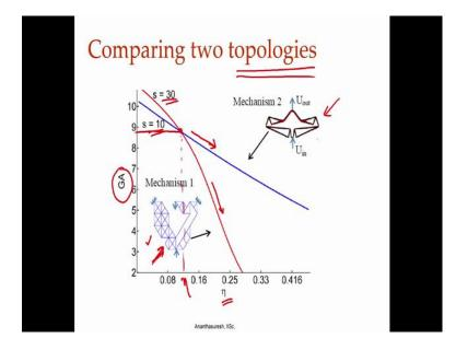
Using these maps if you do it for 2 different mechanisms and put it in the same plot, here of course, the blue one is done for s equal to red is for s equal to 30. So, that they are in the same eta range.
