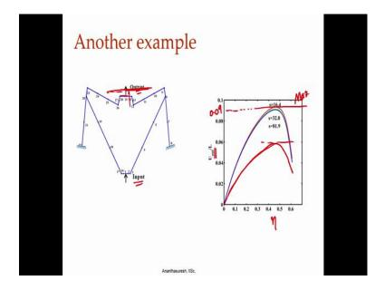
Let us look at this one here is a mechanism where there is some input, there is some output. In this case output by L is drawn for eta, we can see that it an increase it is a maximum value and then comes down so there is a maximum value. Different s values here s is 16 32 and 82. So, the spared is small that indicates that this has little in influence of axial deformation this particular complaint mechanism more than that that it has a maximum. If I look at the value it is let say 0.09.
