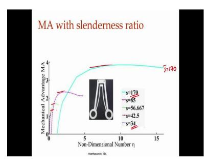
And we can also plot for this mechanism that is the same as what we have here. For different values of a starting from 34 to about 170, this that there is a maximum that things does not change, it is there and you can draw that and see as you increase s value this is s equal to 170 or S bar, it goes to 4 otherwise it is smaller. So, we can get all of this information here.
