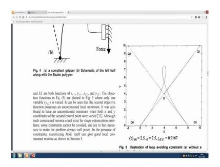
A loop has to be avoided in a compliant mechanism that does not make sense because eventually we are going to make it out of a sheet of material there is a continuum thing. So, having a loop like this would not be referred but there is fortunately a constrained that we can put, what can be called Loop Avoiding Constrained, that again comes from the geometric modeling literature and we can put a length constraint also, we can put a overall how much lengths.
