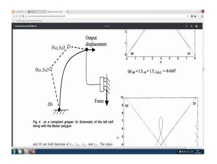
So, let us I want to make a gripper this is a symmetry boundary condition here force is applied when I do that, output displacement should be here let us say gripper problem and I have identified two segments, there is a segment 1 and there is a segment 2.
