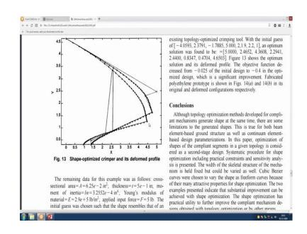
So another example that is shown here again two segments, control polygon for that control polygon for this and here is the optimized one before and after deformation along with the control polygons that are given and this is the one that is fabricated proto type.
