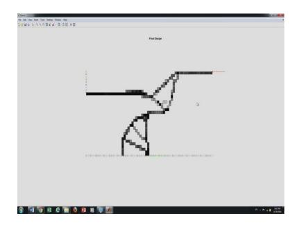
So, now it has done it is job all ready that it came up with a topology like this now what are we doing applying a force here we want this point to move that way instead of a component in that direction not saying that exactly it should moving that if you say exactly should move you put a constrain that it cannot have y displacement which you have not done. So, when this point moves it will have a component in the left direction.
