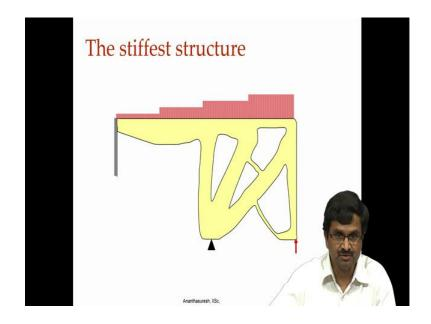
From which we can do some processing to get a structure that look like this, we had done you got a solution for us right, similarly can we apply this technique to compliant mechanisms is what we want to talk about.
