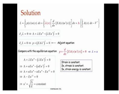
We can do this and solve the problem an electrically and where we can interpret optimal designs as some of the equation show there, show here. We can get a design in this particular case a thing that looks like this area of cross section is optimal one.
