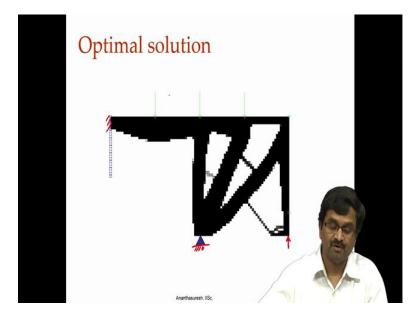
But here do not need to assume anything; we will get the design automatically from the algorithm it looks like this. It says that you have fixed here and there is fixed here right with the load that is over here and the distributed load over there with structure right away.
