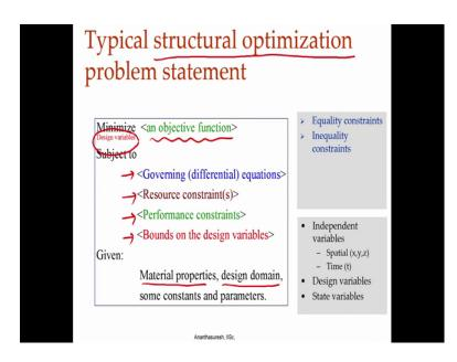
If we take this view, then we can pose an optimization problem when you take structural view point structural optimization naturally comes in where we can have an objective function, we had listed objective functions for a structure similar thing we can do for compliant mechanism as well as we well do later. Subject to some constraint governing constraints, resource constraints, such as the cost material available and so forth, and
