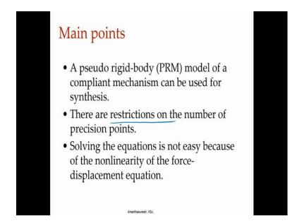
So, to summarize pseudo rigid body model can be used to synthesis as compliant mechanisms, but the trick is here is to identify the number of positions for which we can synthesis the linkage and we will have force displacement relationships as well as loop closure relationships; we have to look at those equations and then see whether they are coupled which one of them can be solved and which one of them should be free choices and based on that we can get this.
