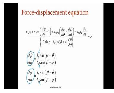
We are looking at this Force-displacement equations and recalling what d b by d theta, d psi by d theta are see this 1 2, 1 3 are there and 1 4 there are the magnitudes of the unknowns that we have Z2, Z3, Z4. We have to see how to manipulate this equation so, that we will be able to get that in a fashion which is the easiest to have them linear then we can solve them happily.
