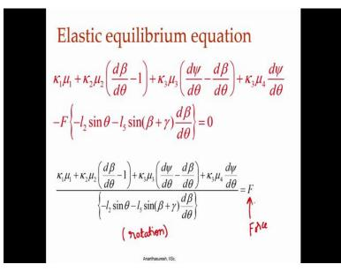
Elasto static equation which is equilibrium equation or force displacement relationship on the right hand side we have the force and on the left hand side we have rotation which is the displacement here. So, we need to find this rotation theta on which the psi and beta also depend. So, we have force and rotation equilibrium equation for the example we had considered in the analysis case you will have this elasto static equilibrium equations.
