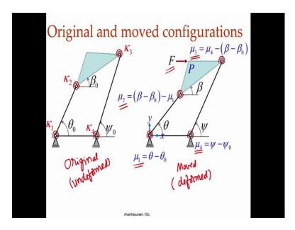
So, let us recall that when we have a compliant mechanism; let us say in this case we have taken a 4 bar linkage, which has torsion springs at it has 4 joints and we want to see if we can synthesis a mechanism such as this for giving specifications of some functionality. So, when we have a 4 bar linkage with 4 torsion springs we already understand that it is a pseudo rigid body model of a compliant mechanism; a compliant
