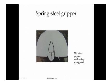
As already showed this mechanism, which is made of a spring steels strip, very thin strip, which was cut with these beams which are 150 or 170 Microns in width, here we can make with metal also grippers.
