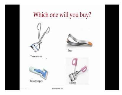
And there are number of products some of them are rigid body linkages here, this is the same function this is the eyelash curler, there is a rigid body, design there is a partly compliant design, there is a flexural joint here. This one has a little metal part that bends
