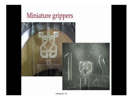
And it polymers of course, you can make many more and here are Miniature grippers you can make a gripper and make another gripper, that can be grafts with the previous one and make it smaller and smaller and you can make the width of this to the limit of what lithography, portal lithography will allow you and which in our lab we go down to 5 Microns very easily, these one of the larger grippers as large as the one in the and the 1 rupee Indian 1 rupee coin.
