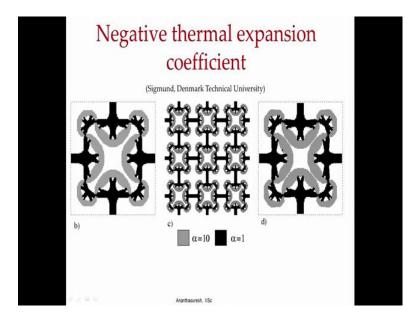
Here is another example unusual property, where there are 2 materials that are used one of them has 10 times thermal expansion coefficient as oppose to another one, as compare to another one this has let us say unit, this has 10 times thermal expansion coefficient alpha.
