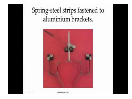
So, we can make very stiffens and we can make compliant mechanisms with spring steel strips, not just polymers you can use any material here aluminum brackets are there over here and here otherwise spring steel strips here, here and here are the ones that endow this mechanism the elastic flexibility.
