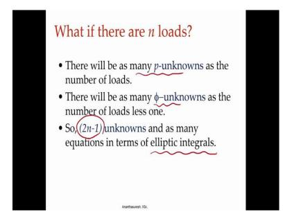
So, if have let us say n loads on a cantilever beam there will be as many p unknowns as there are the number of loads and number of phi unknowns will be one less because for the last 1 phi equal to pi by 2 will be 2 n minus 1 unknowns we have that many equations in terms of elliptic integrals and we can solve.
