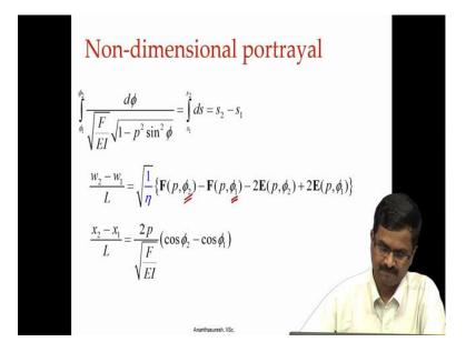
Now, this h is given by this one which you had also derived in the last lecture. Nondimensional portrayal, if I take two different angles in that curve phi 1 and phi 2 the difference in the w direction x direction are given by these two equations again the angles here that we have taken that is where they figure in the elliptic integral solution.
