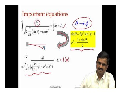
Let us first look at the important equations which are shown here, the first equation shows how the length of the beam is obtained by integrating in the theta of variables.
