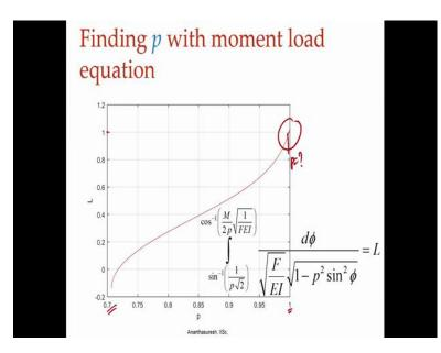
So, we can see it varies p from 707.707 and 2 1 and length is here and it go here that is will length equal to 1 at find the corresponding P value this so close to that this part we will zoom in and try to see and it becomes 1. So, here is where it became 1 and then have to find the corresponding value of p which is 0.9984, it is very sensitive at go up to four decimal places to get it right and you can see that it is only the fifth decimal place that is changing.
