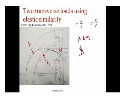
So, what we have here in this case would be an equivalent force P which is equal to the sum of two forces that are applied on these beam P 1 plus P 2 for this portion for this Elastica that calls these there is a modulus P 1, for this Elastica there is a modulus P 2
