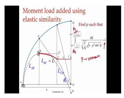
That is if I go back and see this now we have to find p in such a way that when I go from phi B that is what this is to phi C is I go from here to here along this thing here when I do this elliptic integral of the first kind I should get back I again we are given I we have to find p here, P is the unknown for every Elastica here is this characteristics modulus p that decides the elastic is going to look like and p there p end load and that can of decides everything here.
