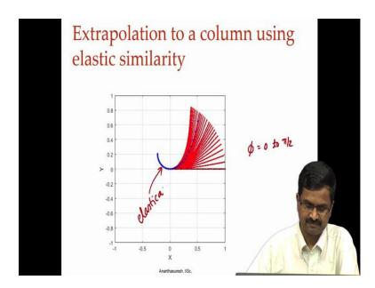
So, as we vary phi from 0 to pi by 2 we get this entire curve for some force values the other one it is a different one that will be accordingly some other curve which we call elastica curve and this elastic similarity is in exploiting this elastica curve.
