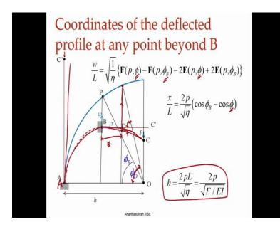
Now, if we look at the geometric significant of that phi when we change the variable theta to phi we know that is the angle that is shown here for point B we go up to p and then connect that gives me phi B. So, only for point D B go there and point C phi equal to 90 degrees because if a go up and come down and look at the angle that is 90 degrees and for this point which had called A earlier phi is equal to 0.
