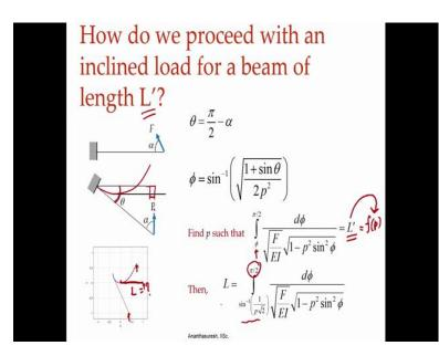
Now, if we see in general; if you are given a beam of length L prime and the load is given at an angle alpha how do we proceed in order do that what we do is we have to imagine that we have to turn it around. So, the beam inclined load should be like this. So, that we get the equivalent beam which is horizontal and that has a length L we want to know what that L is for that what imagine that we rotate this beam.
