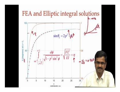
This is with the finite element cod, now from the finite element code we have gotten d theta at the fluent that is; if I have a beam when it is going to bend like this when we apply force there this here is theta L that is shown in this blue curve this is finite element solution.
