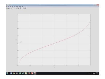
Here we have plotted l verses this p when l were as is 1 meter. So, 1 is over there. So, let me zoom in to see what p value that we need to take. So, if I what to zoom in around 1 this is graphical way of solving an equation were we know the right and side we are get the modulus of the elliptic integral write do this few times then I would get that.
