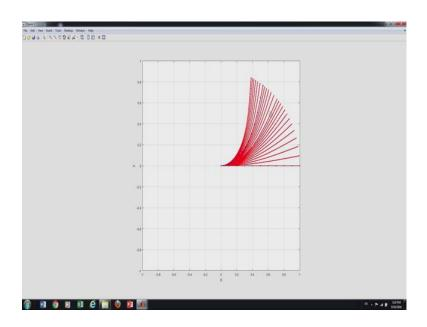
Here is the code that illustrates elliptic integral solution for large displacement analysis of cantilever beam; it uses non-linear finite element beam code written by my student P
