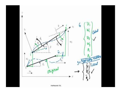
So, if let us look at this particular one here the original beam is here. So, this is the original beam segment let say we have an elastic segment in a complaint mechanism we have isolated one of them there are 2 nodes 1 and 2 this is the original configuration, after the complaint mechanism deforms let us say this original 1 2 has gone to let us say 1 prime and 2 prime, that is node 1 has gone to this node 2 has gone to that point.
