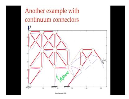
So, here is another mechanism that also has lot of this connectors were the blu e lines are the deformed ones this is deformed and the red ones is undeformed and again it compared well with finite element analysis of the continuum elements.
