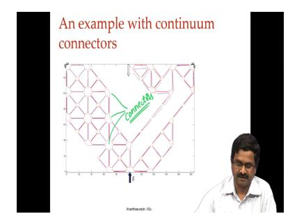
So, these are all the connectors we see lot of them wherever beam segments meet we can make this connectors now, this turned out to be more accurate and closer to the real device which is analyzed using continuum elements, another with beam elements is simpler and it is preferred, but continuum elements are always more accurate and here the beam elements are fine, but the way we model them is different. So, we decided that we need to have these connectors there. (Refer Slide Time: 24:57)
