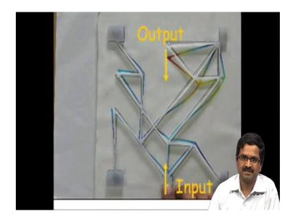
And the kit these example we showed when you have input and output here with the red ones where it is it was fixed and if you push it; it is coming down note how it deforming and then we will see the continuum version it deforms exactly the same way. So, you can conceive a compliant mechanism using this rigid connectors where you can have snapping beams going into it.
