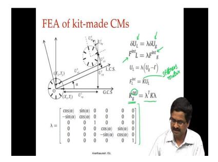
So, lambda little close up to use you can read the things better this rotation matrix is there is a incremental displacement delta U L and delta U g and delta U L are related by this rotation matrix and so are the internal forces will be two forces in x and y directions as well as moment that will be there in this vector. So, global coordinate system forces local global system forces are related again in the same rotation matrix and this one we talked about U L and U g how they are related.
