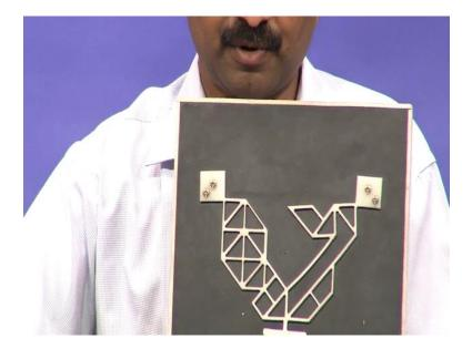
So, I can look at something like this identify all the nodes and all the elastic segments and know the cross sections with depth and breadth known then I can put it in the finite element code then I can analyze as we have shown.
