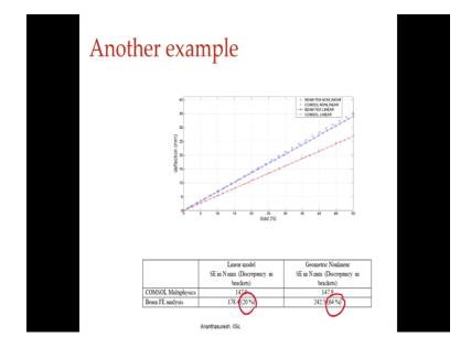
The quantification when you do it that is when these errors will be apparent and here is another example that is based on a different mechanism that I do not have which mechanism it is, but here the error is 20 percent and 64 percent. Sometimes the errors could be low, but even 20 percent we cannot tolerate, sometime maybe only 5 percent but the problem exist the way you model a mechanism is causing this error and that has to be fixed.
