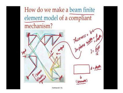
If you look at the mechanism that is shown in the slide, if you look at this everything is like a continuum in fact, what we have done here is we have taken a sheet of polypropylene and using CNC machining have cut out a lot of holes that you see this is this triangular thing is a hole, this
