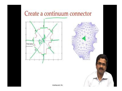
So, this connector that you see is rigid one with all the fillet radiate taken and that is modeled as rigid element along with beam elements. So, if there were to be eight things meeting at a node such as this they all have different widths. So, this width is more than this width and that one is more than this and everything has different widths here is where the beam elements go. So, a beam element goes there, goes there, goes there, goes there and so forth.
