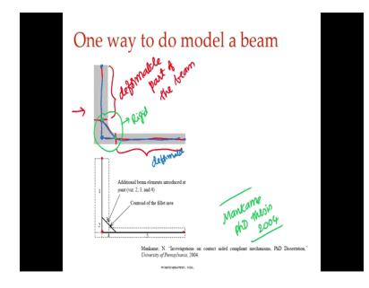
So, one way to deal with this situation is that when I had a realistic structure that looks like this. So, I have a compliant mechanism that has segments like this now one way to model this is to have a node there and a node here and a node there, that is I put a node and a node and a node there, but the fact that there is so much more material at the center and the effective length of the beam.
