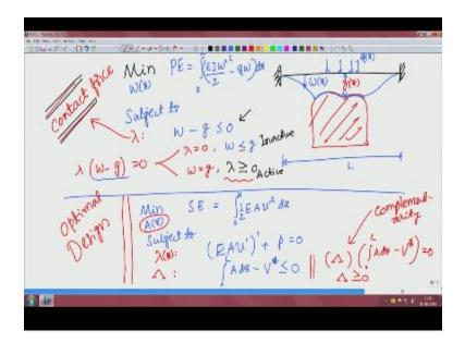
Let us I have a beam which let us say is fixed at both ends and I have a rigid obstacle of some kind here okay there is a rigid obstacle okay now when this beam deforms it cannot go through it so there it has to follow the profile when there is some loading that is applied on this say some Q of X okay then it has to follow it cannot go into this obstacle so it where it has to follow this so
