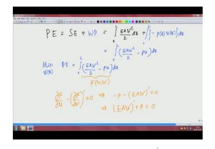
Here external force is that P external forces okay so what we have here if we write for this problem potential energy is strain energy plus work potential we just derived the strain energy let us actually right in two different colors so we can easily see which is which okay so they say strain energy we already wrote 0 to L EAU prime square by 2 DX and then work potential plus
