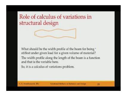
In the case of structural design let us take the same beam fixed on both side sit cross section area profile can be different from point to point this is not how we see normally beams in any room there will be uniform cross section okay but one can make variable cross section beams and that is a structural design problem there what is an unknown the area of cross section a of X if I say these x axis from 0 to some value L A of X is an unknown function.
