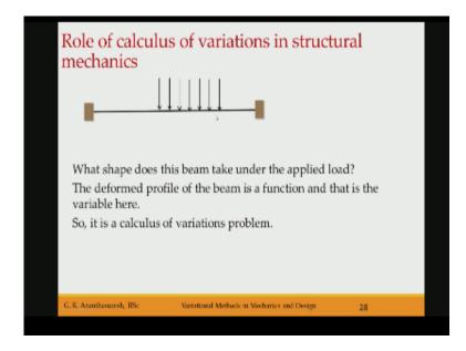
Let us look at these variation methods in mechanic's first okay so if you have abeam like this which is fixed on this side as well as on this side there is some loading on it, it is going to deform and take a deformed shape okay the beam has the freedom to deform to any shape but it does deform to a particular shape because that particular shape minimizes the potential energy just like we saw a spring with a mass it displaces by a quantity which minimize the potential energy.
