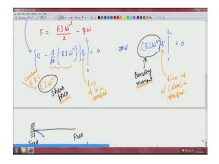
When W specified surface is equal to 0 in this case the shear force need not be 0 it can also be 0 in special cases in generally not be 0 similarly w' slope is specified by cantilever beam over here then the bending moment need not deserve it can also be 0 but need not be 0 okay but if it is free w are specified then the shear force should be 0 at this point and show so should be the bending moment both shear force and bending moment or 0 here okay.
