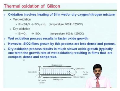
One of the easiest film that can be made on a silicon wafer is the oxide of silicon, and it can be fabricated in a simple furnace like this by processes known as oxidation and when whether there is you know steam present or not we call it wet or dry oxidation method. And the Chamber that you see here is a dry oxidation furnace in which you have gas outlets. And there is a series of wafers assembled.
