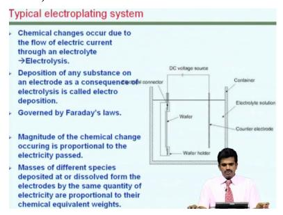
Changing gears one of the simplest approaches and probably the most widely known approaches is based on electroplating, sure you would have heard about this in various other context, what you would require is an electrolyte bar in which you apply a potential between the cathode and
