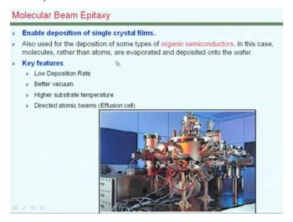
Then one more you know although not very much used in the context of microsystems per say, but even higher control of film characteristics can be obtained by an approach called Molecular beam epitaxy, where you know which is also a very low deposition scheme and as you could see from here a highly complex kind of a system used quite for this purpose as well.
