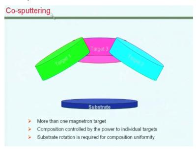
In this approach it is also possible to do a Co-sputtering with multiple targets, so when we need a composite film it is also possible you know locate these targets appropriately, so that we can have a Co-sputtered film which will be based on the various materials that are provided with individual targets, so that is one key advantage of using sputtering.
