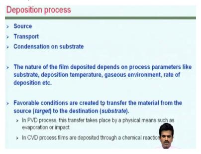
But oxidation is only possible in the case of silicon and only to form silicon dioxide, in general to deposit to work with thin films we need to start with the source material of the thin film and transport this source material and deposit condensate on to the substrate. So a series of process steps would be required in a general scenario when one would want to deposit a thin film onto a wafer whether it is silicon or other materials.
