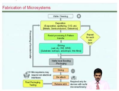
As we have seen in the previous lecture, one of the key steps in the whole chain of events that are required for fabricating microsystems is essentially deposition and this is done by various methods and various different materials can be you know fabricated by that methods that you will see in today's lecture.
