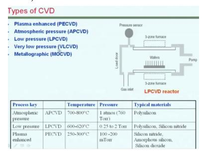
So one you know typical situation in which the films are formed on multiple wafers is shown here, we how to control the pressure inside the chamber temperature and various parameters. And there are various types of CVD based on how we enable these chemical reactions to happen, there are techniques in which we use plasma inside the chamber and which is usually at lower temperature, there are also methods in which lower pressures are used.
