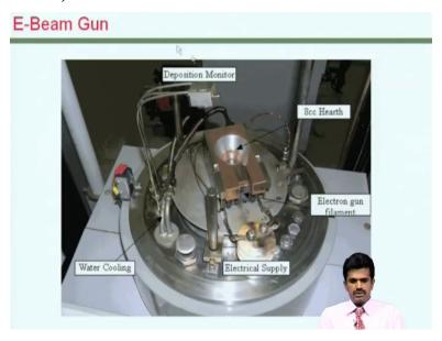
And what you see here is an image of an opened out chamber in which this electron beam gun can be seen very clearly.
