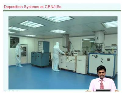
What you see here is set of deposition equipment that are available at IISc where you know we can use sputtering or evaporation kind of techniques for depositing various films.
