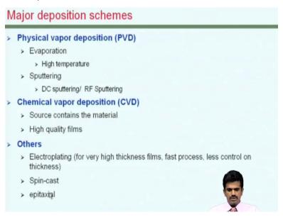
Major depositions themes therefore, are based on either they are physical vapor deposition or chemical vapor deposition. In some examples of physical vapor deposition includes the evaporation technique and what is called as sputtering technique, there are several variants of these as we will see in subsequent discussion. There is also as I mentioned chemical vapor deposition techniques which is typically used for better quality films.
