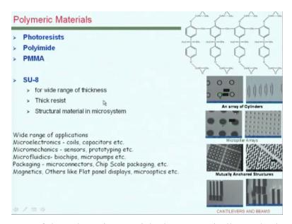
So let us look at some of the polymeric materials that are typically used. Photoresist is a resist material and as you will see soon in another lecture, this is required for the pattern transfer in most instances. Polyimide and PMMA polymethyl methacrylate are very common materials plastic materials, polymeric materials used in various microsystem applications. As I mentioned SU8 is fast becoming a another popular polymeric materials which can have a wide range of thickness.
