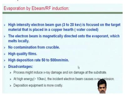
It is also possible by you know RF induction by to generate such beams which could essentially displace these atoms from essentially the source material inside the crucible and these approaches would result in relatively better quality films compared to the simple heating based approaches, and have reasonably good deposition rates. But you know because this includes
