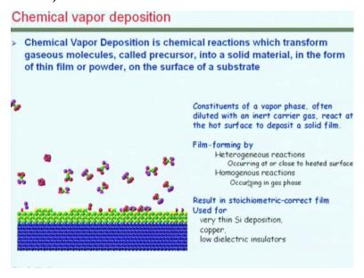
The next deposition approach that we want to discuss is based on chemical vapor deposition, so in this case a chemical reaction would happen which would transform the incoming gaseous molecules which are typically called precursor, and we make them you know after the reaction the precipitate of the chemical reaction would be made to stick onto the surface. So in this case there are no real target, it is essentially incoming is the gaseous form.
