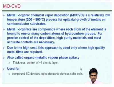
It is possible to deposit metallic films also by CVD techniques and typically these are called MOCVD Metal organic chemical vapor deposition schemes, so what we have is that precursor material is typically metal organic of the particular metal to be deposited, this results in extremely high quality films and you know but at very low rate of deposition. Hence it is used
