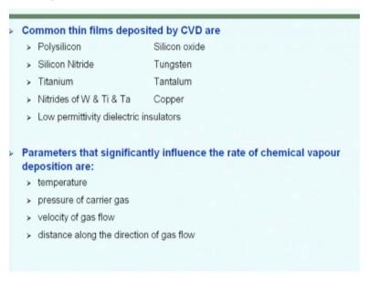
Films include the silicon compounds, metals and also various other dielectric insulators. The process parameters include the temperature, the pressure and the flow of the gas and the distance on within the chamber and the direction on which these are incident on to the surface.
