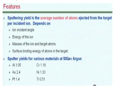
There is a terminology called sputtering yield which is essentially the average number of atoms ejected from the target which is kept at the cathode and that will depend on the incidence angle for the ions, the energy of the ion, the mass of the ion and the target atom and the surface binding
