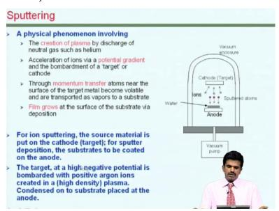
The second physical method that listed there is sputtering, so this is once again a physical phenomenon of transporting and in this case it is done by creating a plasma and the ions created by this plasma are attracted towards the positive ions are attracted towards a cathode and the source material is kept at the cathode and these ions when they bombard the target, the atoms from there are sputtered out and we keep the wafer at the anode.
