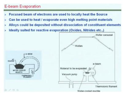
But you know most materials have much higher temperatures and cannot always be melted just by heating them, so we use other ways of energizing their atoms or molecules from the source, so that these could be displaced and transported onto the substrate surface. What you see here is an arrangement in which an electron beam is used for evaporating the source materials inside a crucible and this could be you know directed towards the wafer carousel.
