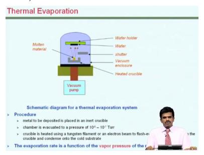
Let us first look at this example of thermal evaporation which is usually done within a chamber like this. Let us look at one of the common examples of evaporation that you would have seen in your own house one of the common example is basically you would have seen water boiling in a vessel in the kitchen and if you put a cold lid over the boiling water, you can see that the water condenses on that lid surface.
