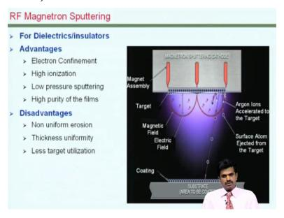
The essentially 2 types of sputtering depending on how one creates the plasma, can create a plasma with DC for conducting materials such as metals we create an RF Magnetron based plasma for dielectrics or insulating materials, and that has better control especially for you know depositing dielectric materials, and once again this is also very popular you know large area films especially for industrial applications.
