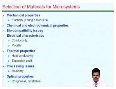
Now we can also look at how these materials are chosen for various applications in microsystems especially in the context of microstructures one would want to primarily look at the mechanical properties, the elasticity, the Young's modulus of the material, and as I mentioned that depends on the material per say as well as how it is deposited. The chemical and electrochemical properties of various materials are relevant.
