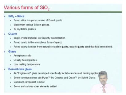
There also several forms of silicon dioxide which are used in microsystems, silicon dioxide can be used as you know as a thin film, it is also used as a substrate material in various context for microsystems. And various silicon dioxide is also the constituent of glass and various forms of glass are also used in microsystems. So what we have seen in this lecture today is a several set of
