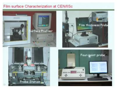
The film characteristic that I have mentioned are evaluated using various instruments that are shown here. The thickness as well as the uniformity of the thickness can be evaluated using a surface profiler, what you see here is a contact type surface profiler, where there is a scribe which would actually move and its position is recorded, and based on deposition of this tip of the scribe one can determine the height of the surface of the film.
