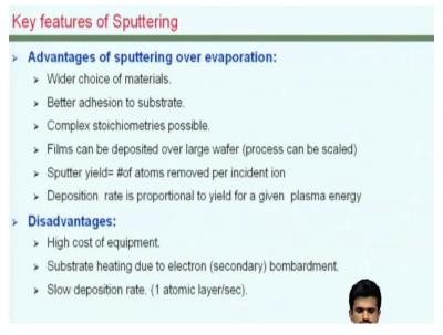
The basic features of sputtering includes you know the wide choice of materials, because in the case of evaporation if you recall you could only have materials which have relatively low melting points. And since the sputtering is done usually at a lower rate they have better adhesion characteristics and there are ways in which one can engineer the sputtering to have complex stoichiometric you know make films.
