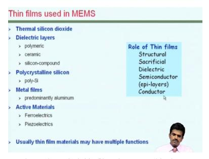
Let us also look at you know the typical thin films that are used in the context of microsystems, as we have seen in the beginning thermal oxides of silicon is a important component in this context. There are various dielectric materials other than silicon compounds that could be used in microsystems and this includes polymeric materials some of those I have already discussed.
