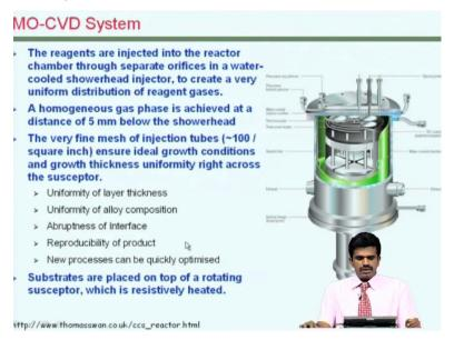
In a typical MO-CVD system variously reagents are injected into this chamber and just like in any other CVD scheme you know we make the chemical reaction to happen, and we also do some kind of rotations and things like that, so that you know a uniformity and good control of the film deposition can be obtained by this approach.
