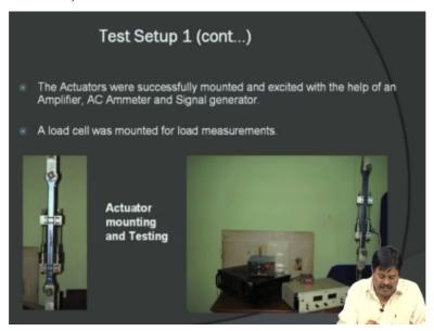
The actuator was loaded here with the bracket here and this is the strut and the experiments were performed in the laboratory and the load cell was mounted for the load measurements in order to find out the levels of the load coming here.
