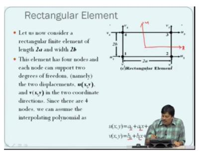
Now let us go to a 2 dimensional element and suppose we have a rectangular element of length 2a and width 2b, which has 4 nodes and each node can take 2 degrees of freedom that is u and v in 2 horizontal directions so it will have totally 8 degree of freedom element. So we have 4u degrees of freedom and 4v degrees of freedom that means the polynomial is not only x it is also y dependency is there.
