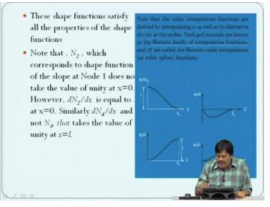
These shape functions essentially satisfies the properties of the function and I have specifically said that N2 which correspond shape function of this slope and node 1 does not take a value of unity at x=0 even though it is evaluated at that node, only dN2/dx=0 and if you plot this you see that the variation, N1 takes the value of 1 and 0 at 2. The slope dN2/dx takes the value of 1 at node 1 and 0 elsewhere.
