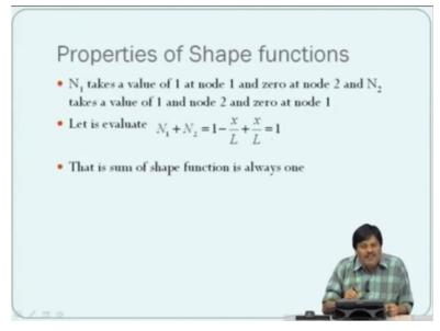
So the sum of shear functions are always equal to 1. So these are some of the properties of the shape functions. It takes the value of unity at the node where you are evaluating it the coordinate and all other places it is 0.
