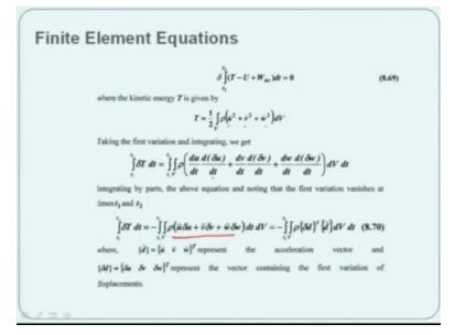
So now let us begin the finite element equations. How do we get the finite element equations? So we again talk about we go back and revisit our energy theorems and one of the energy theorems we derived is the Hamilton's principle because we are now trying to derive the equations for the general dynamic equations and then remove the dynamic part of it and solve only for the static part.
