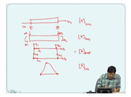
So the rod problem basically will have 2 degrees of freedom that is the axial displacement u1 and u2 and this is node 1 and node 2. So in this case, the stiffness matrix k which we represent will be 2/2. If the same problem is now a beam problem that is when the loading is in the transverse direction in this direction, then it will take 2 degrees of freedom that is the w1 and theta 1 the slope and w2 and theta 2 slope.
