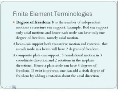
So now let us introduce certain terminologies. Degree of freedom, what is degree of freedom? It is the number of independent motion a structure can support. Example, a rod can support only axial motion in the 2 nodes and hence it has 2 degrees of freedom. It is a number of independent motions. For example, a beam can support both transverse motion and rotation so that is each node in a beam will have 2 degrees of freedom.
