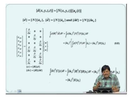
So before we do that now we said that in finite element we assume the variation over each element. That is the variation can be expressed in terms of the shape functions, which I talked about in the first slide multiplied by the an of t, the an of t is the elemental displacement vector of the element, which I call it as ue of t. For the sake of convenience, ue means e is the elemental vector whereas u is the global vector.
