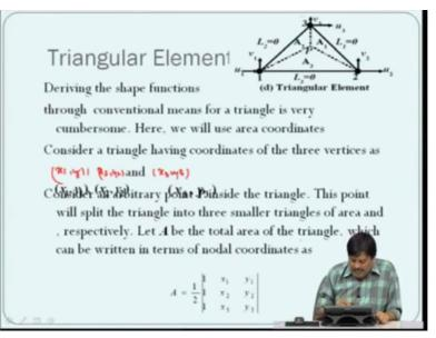
Now for the triangular element, how do we do it? So now let us look at it is very important element but inconvenient to generate the shape function by the procedure we adopted before even though it can be done. So here we take a slightly different approach where we will not use the conventional coordinates, which is given by you have x1 y1, x2 y2 and x3 y3. What we will do here is we will take any point for which we require a coordinate.
