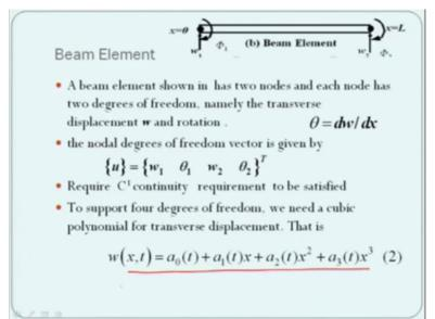
We will do the same this with beam element. As I said the beam element has 2 degrees of freedom for node, which is w is the transverse displacement and theta is the rotation. So the minimum order that is needed here is it has to have 4 degrees of freedom are there so with the
