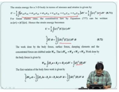
Next, we take the strain energy part. We know the strain energy, we derive the strain energy for a 3-D state of stress which is nothing but is given by this expression where it is a product of stress and strain in each of these planes, which can be written in matrix form in this form and when we take a variation we have to take a variation on displacement or the quantities
