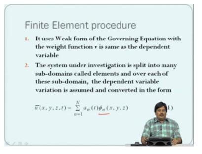
We said that finite element uses the weak form of the governing equation with the weight function v which is same as the dependent variable function, which is given in equation 1 here. So the system and the investigation is split up into many subdomains, which we call it elements and each element has a number of notes. Over each of these subdomains, the dependent variable is assumed in certain form of a series, which is given by here equation 1 where an of t and phi n has certain meanings.
