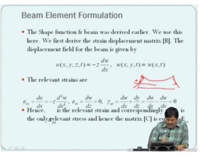
Similarly we can do the beam element formulation where we have the displacement relation between the axial displacement is given by theta times slope. So basically when the beam bends we have so this is the mid plane so we draw this and this is the axial displacement, which is the theta so that is the z times theta is nothing but the axial displacement and this one.
