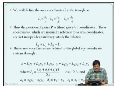
So now we will define the area coordinate for this problem or the point P it is located by L1, L2, L3 where L1, L2 is the sub area A1/A so if you look at it the sub area A1/A is the L1, L1 is the one where the opposite node is the node 1. Similarly, we take L2 which is the sub area A2/A, L3 is A3/A. The position of the point is thus given by these coordinates, which are normally refer to as area coordinates and or not independent and they satisfy the relation L1 L2+L3.
