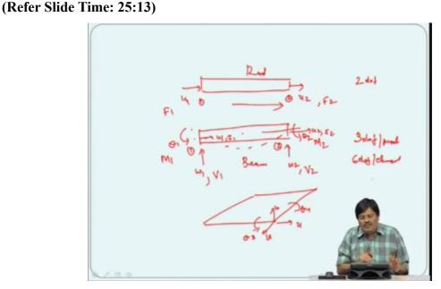
To explain this a little bit, so let us take a rod. So rod can move only in this direction, it can move only in this direction so basically that means you have 2, this is node 1, this is node 2.
