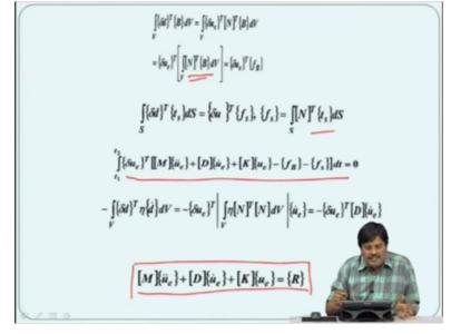
So this can be written in this form mathematically. Similarly we can write the body force delta d using this expression here we can write a delta d transpose is delta ue transpose into N transpose and multiplied by the body force vector and this is the discretization of the body force. So this basically converts the body force, which is distributed into the concentrated force acting on the nodes.
