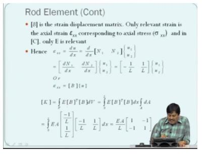
So B is the strain displaced only relevant strain is epsilon xx. So only you will have C present here then we put the C back here. So once we use this we can actually get the strain displacement matrices and the C matrix will contain only E the Young's modulus. We substitute all these things into this equation replace C/E, once we do that we get this equation.
