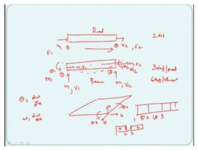
That is for example if you have a series of rod element and we isolate it, this is element 1 and element 2. So the element 1 this will have 1 and 2, 3 so the axial displacement 2 due to element 1 should be equal to the axial displacement at 2 due to element 2. That is not at all an issue because it can be maintained, but if it is a beam normally in beam the slope theta here is derived from dw/dx from the transverse displacement w.
