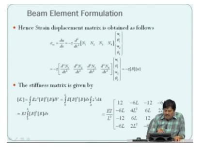
Here we plug this back into this equation and derive the strain displacement matrix, which is du/dx which is given by there and when we substitute for u we get this is the second order matrix and we substitute back into the governing differential equation and integrate between 0 to L we get this is the governing equation.
