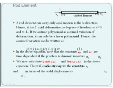
For example, if it is a rod problem, so for the rod problem we basically have the element has 2 degrees of freedom x=0 and x=L, so if you want to approximate the variation within the element and use polynomial we need to have 2 unknown constants into the variable that we
