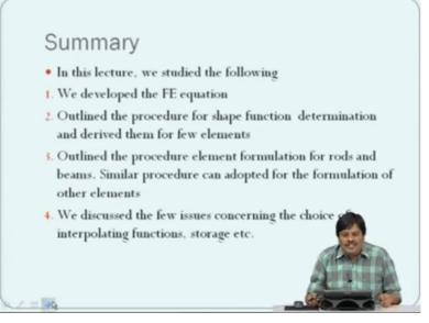
So basically we have done this and now in summary what we have understood here is we have developed the FE equations, outlined the procedures for finding out the shape functions and also derived some of the elements that can be directly go into our analysis like rods and beams and we also discussed few issues concerning the choice of the interpolating functions etc. Thank you.
