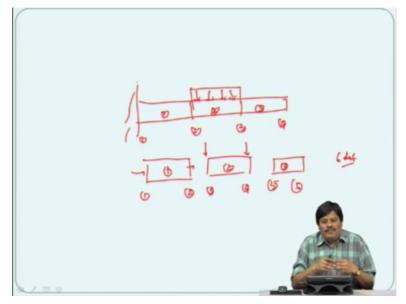
For example, if you have a structure say we have a rod where some portion is having some distributed loading. So in the finite elements, we can only handle concentrated loads. So basically we split this element into sub elements so this will be element 1, so this will be element 2 and this will be element 3. So I will name it as 1, 2, and 3. So each will have say 2 degrees of freedom.
