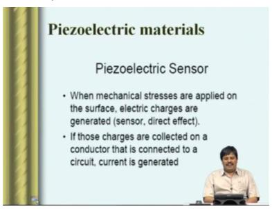
But if I want to do the inverse effect that is when I want to use a piezoelectric material as an actuator here when an electric potential or a voltage is applied to the surface of the piezoelectric material, the mechanical strains are generated and if the piezoelectric material is bonded on to the surface, these strains are applied to the structure and the forces are
