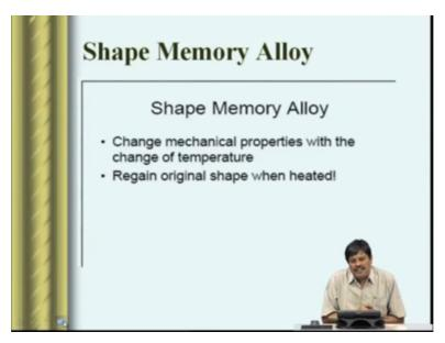
The next material what we are talking is the shape memory alloy and the shape memory alloy basically changes the property with the change in temperature. So basically in the normal temperature, it will be in one phase. When the temperature increases, it goes to the other phase and retains the memory that is precisely it regains the original shape when heated.
