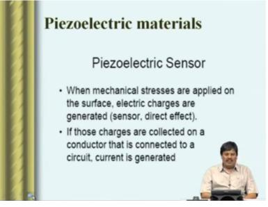
So as I said earlier in a piezoelectric sensor, when a mechanical stresses are applied on the surface, the electrical charges are generated because of this sensing effect and these charges are collected on a conductor and that is connected to a circuit and a current is generated. The current gives out a voltage signal, which actually states the state of this particular structure.
