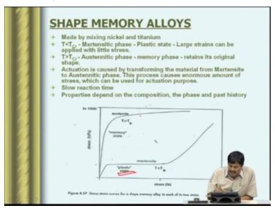
So if we look at it, in the normal temperature the material is highly plastic, which is shown here. This is a very plastic state then it goes here, but when the temperature increases it goes to the austenite phase. Suppose we actually prevent it the amount of actuation force available is enormous, the amount of stress that is available is enormous, which can be used as actuation.
