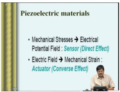
So this is what is given here. So the mechanical stress are generated, the mechanical stress inputted into the system generates an electrical field, which is called the sensor effect as I said earlier it is called the direct effect and whenever you feed an electric field and it generates a
