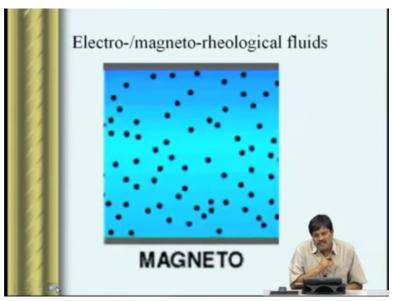
So basically you could see that in this video, how the material which was arbitrary were oriented due to the application of the field. So this clearly says by this process, a fully liquid becomes a semi solid material. So basically it is a smart material that can change the viscosity thereby it can be used for applications involving damping of the structure.
