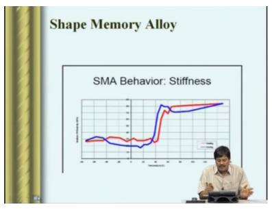
So as I said the stiffness of the material changes with the temperature. Here there are 2 things, the blue is basically tells when it is cool and when the material is heated you see the young's modulus changes. So this change in the behavior of stiffness can be very successful in using for the actuation, but the main disadvantage here is its reaction time is very, very slow.
