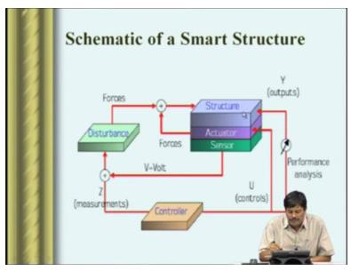
Next we will go and find out what is a schematic of the smart structure? So basically a smart system or a structure would have a structure, it has a structure. The structure has actuator, a sensor. So basically whenever there is a disturbance that is given to the structure, it can be like a force. If it is a piece of sensor, then the sensor will measure the strains in the structure and give out in the form of a voltage.
