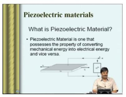
Let us begin with the piezoelectric material. What is a piezoelectric material? So piezoelectric material is the one that converts the mechanical energy into electrical and vice versa. So basically here there is a diagram. There is a structure with the piezoelectric film there, which is pulled here. So when you apply a voltage, it generates a strain and when you induce a strain through a force, it generates a voltage.
