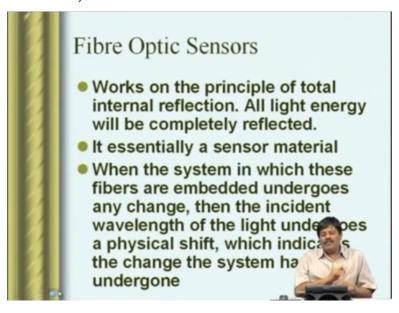
Next, we will go to the fiber optic sensing. Here the fiber optic sensor is basically works on the principle of total internal reflection. In the total internal reflection, all the light energy is reflected without any reflections. It is basically a sensor material, fiber optics cannot do any actuation. So how does it work? When the system in which these fibers are embedded undergoes any change then the incident light has a wavelength and that changes when it comes out.
