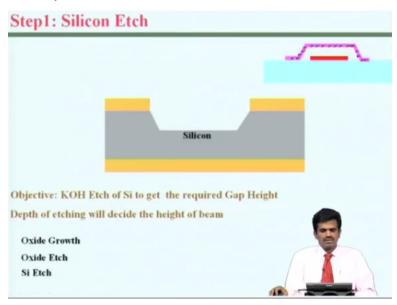
To do that will actually start with a silicon wafer and we will do KOH etching which is essentially anisotropic etching to create this height on silicon wafer. So eventually the silicon wafer is going to sit on top of this glass wafer and we will bond them together. So the depth of etching will be decided how deep, how high this beam would eventually be.
