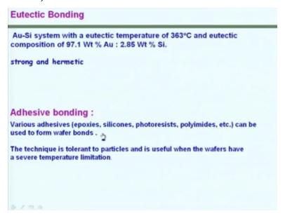
Another approach that is often used is known as eutectic bonding in this case a thin layer of gold is used on top of the silicon to essentially enable this bonding. The temperature is of the order of 360 degrees with the kind of right; basically the weld material has the composition as you see there. And the next approach is by adding an extra adhesive layer of various types like epoxies or polyamides which could you know create bonding between this at relatively lower temperatures.
