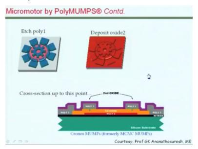
So essentially it is a series of oxide and poly deposition and patterning and you know if you go continuously like that we can create you know this rotor and stator structures on top of this silicon. So by you know obviously one may need to take protective steps in the process so that you know unwanted layers are not removed. So we essentially have these 3 layers of poly poly0, poly1 and poly2 which would be used for constructing these geometries vertically.
