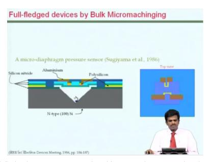
Now look at full fledged pressure sensor using this approach. You see that there is a diaphragm kind of geometry here and then there is this cavity below that. How do we go about building this? As you see we need to build all these thin films, we also need to create this cavity, we have seen that cavity like this could be built by bulk micro machining. You have seen that all these layers could be added by this series of deposition and patterning steps.
