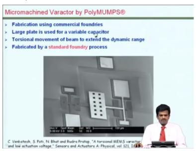
There are also several commercial approaches which could be used for building fairly complicated Micro Systems. What I show here is the picture of a varactor used fabricated using commercial process. As you see here a large plate which is essentially a moving structure and associated with this, there is a smaller plate which would be actually the actuating electrodes in this particular case and you know so fairly complicated looking geometries could be done by this approach.
