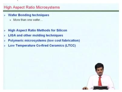
So what we see so far is you know various possibilities with which adding a few layers of poly silicon or other materials one can build fairly complicated microstructures. As we have seen today wafer bonding is a key process that can enable various new possibilities into building Microsystems on silicon. This essentially adds more than one wafer either 2 silicon wafers or a silicon wafer and a glass wafer.
