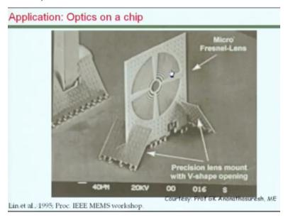
It is possible to make them to stand vertically by slight modifications to the processes and we can even use them in an optical chip.
