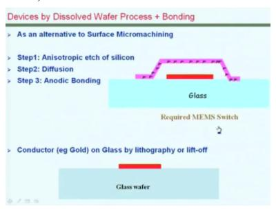
Now we will see how this can be extended to building Microsystems. What I show here is an alternate approach to build a micro switch using a process known as the dissolved wafer process which involved the glass to silicon bond. Essentially happens in 3 steps how we attach this top moving member on to this glass. We obviously start with the glass wafer and then pattern this conductor the red color conductor which could be gold and can be patterned by either lithography or lift off.
