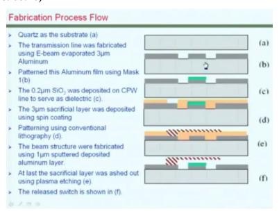
And if you go through the process steps, we can start with the substrate and on top of this first as we have seen the transmission line is fabricated by first evaporating aluminum on to it and then patterning this aluminum. The next step is to use SIO2 to basically add this protection layer that I mentioned and on top of that after patterning this we will add the sacrificial layer to create this
