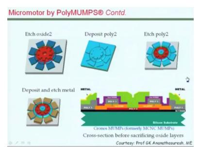
And with the poly2 layer we can create all this stator and rotor geometries as you see it here. On top of it, we can add a metal layer to create the electrical contacts later.
