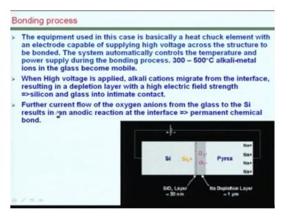
So when these kind of glass that you see there and silicon wafer that you have, when these are bonded together essentially there is some kind of migration of ions happening at the potential that you apply which would essentially facilitate the bonding to happen.
