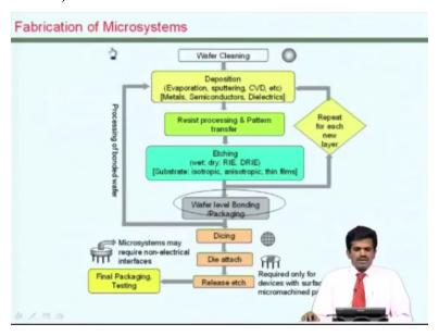
As you see from the flow chart that we have been using the wafer bonding process is one of those steps which is used in this closed loop what I mean to say is that even after it is done first of all while the full wafer is under process, secondly it can be subjected to subsequent processing of deposition and etching afterwards. The question is how do we do this and you may recall this is now a partially made geometry.
