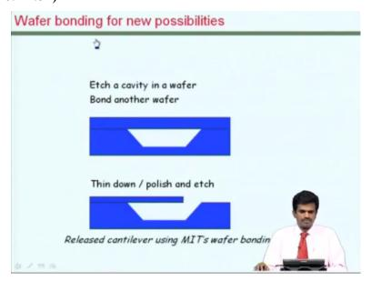
There is an alternate approach to built structures above cavity. And many of those use what is called the wafer bonding process. What can be done is that you create this cavity and the bond another wafer on top of it to create this kind of closed cavity. It can be etch standard for cantilever kind of structures as well. This process as I mention is called wafer bonding process.
