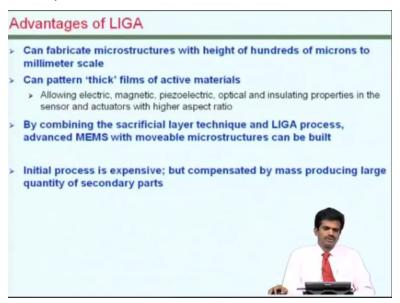
So advantages of LIGA process would be that one can build you know even up to 100 of micron thick microstructures which could be patterned and this can even be combined with surface micro machining and other conventional MEMS based approaches for building really useful Microsystems. The point to note is that the X-ray lithography process which is the first step is fairly expensive, but this is compensated by the mask production of the large quantities of those secondary parts that were formed.
