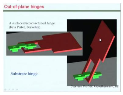
Is it possible to build geometries that can actually know stand vertically. What you see here is you know a schematic of a hinge that has been fabricated by micro fabrication and made to stand vertically.
