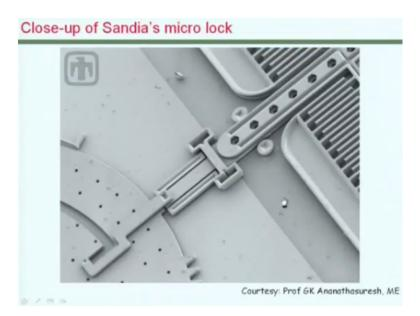
It also enabled multiple layers of polysilicon structures to be form to built complicated looking microstructures as the one that you see here from the Sandia labs.
