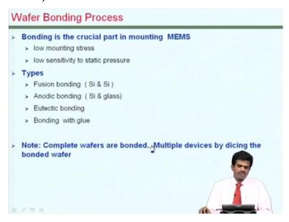
So as you would notice this kind of bonding is the very crucial thing in many Micro Systems. There are several approaches to build bonded wafers of silicon or silicon and a glass wafer or it could be based on additional layer as you would see later in this lecture. One thing that you should note is that this is bonding usually to complete wafers. This is not a part of a device getting added to a part of another device.
