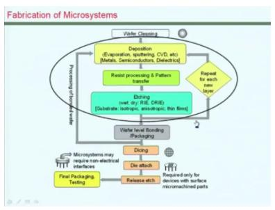
If you may recall Microsystems fabrication involves a series of cross steps, many of them are done within this loops where you have deposition patterning or pattern transfer and then you know repeat those to build useful Microsystems. Deposition schemes involve evaporations, pattering, these are 2 of the physical deposition schemes commonly used. There are several chemical vapor deposition schemes.
