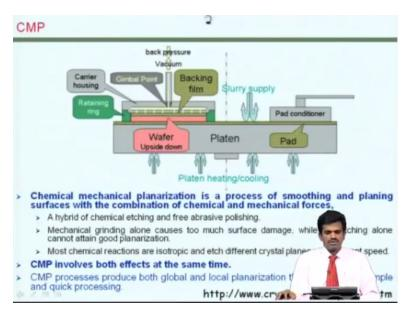
So the process involved would be you know to put the wafer for on a platen which would be rotating and in a slurry which would be chemically active slurry and also which cause the mechanical action mechanical grinding action to happen. So in CMP both those actions will happen together and can be therefore used for quick polishing of the surface of the silicon wafer and this is widely used these days for both microelectronic wafers and silicon wafers.
