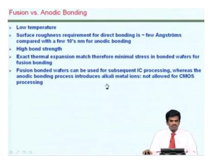
So the surface roughness is a key thing in success of controlling the surface roughness is a key thing in the success of these approaches. These wafers can be used and have been used in IC processing itself and many of the CMOS processes could be subjected to because you have both on both sides silicon wafers.
