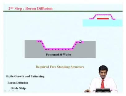
Onto this wafer, we now do boron deposition, a serious deposition of boron and so that it becomes a heavily doped thin layer. So again we do outside deposition and again pattern the outside so that this region is exposed and then diffuse by putting this in a diffusion furnace and then after the diffusion the outside is trapped and how this layer which will be heavily doped region of silicon.
