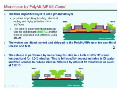
With this after removal of those oxide layers we can create these geometries to be freestanding and the wafers could be used as individual devices by dicing them usually, usually if you recall dicing is done before the sacrificial layer is removed. So sacrificial layer is removed if you may recall by usually by this critical point drawing process if it is used the situation can be avoided.
