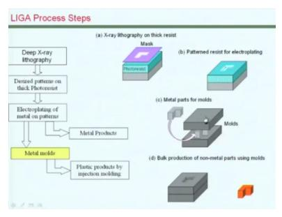
How does LIGA work? We use as I said X-ray lithography, why X-rays? Compared to the optical lithography, this can go deeper into the resist, so we can use the thick resist layer which could be patterned by this X-ray lithography. Obviously the mask that you would use should also be different to enable the X-rays being used for this purpose. So the desired patterns are formed first on this resist. This resist in fact sits on a metalized let us say wafer.
