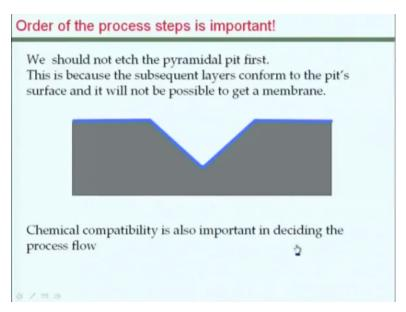
So the thing to remember is that although this geometry you know it looks appealing that we are going from bottom to top. You should not be etching the pyramidal pit first and you should also think about the chemical compatibility in deciding the process flow because if you are using this KOH etching the layers that you how you put previously here should not be affected by this KOH etching.
