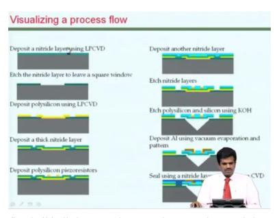
We will basically first build all those top layers and pattern them and then only etch through sideways and etch down towards the substrate. So in this particular case we have nitride deposited and patterned and polysilicon layers added which would essentially work as those resisters which would, whose resistance would change based on the deformation and additional layers and finally this KOH etching the anisotropic etching of the silicon.
