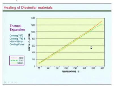
We wonder what would happen if you are to use these 2 different materials, silicon and glass. It so turns out that some of the glass composition that we use for this kind of purpose have the same thermal expansion characteristics as the silicon wafer. So there is no shear force that would happen at the kind of temperature ranges that we are subjecting it into. So it is not a problem from that point of view.
