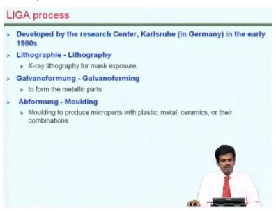
So we will see now how the LIGA which is an approach which is now available for about 30 years could be used to build geometries based on the fabrication approach is that we have seen previously. In involves lithography to build thick layers but different from what we have seen before it then you know uses electro plating and kind of molding of parts to build these extended geometries.
