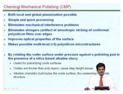
This is essentially used for planarizing the wafers which is partially processed. So as you see here it has both chemical and mechanical aspects of polishing. How do we polish it chemically by essentially etching and we have seen that the isotropic etching of silicon can be used to even out the surfaces. Obviously you all know that mechanical grinding also do the something same.
