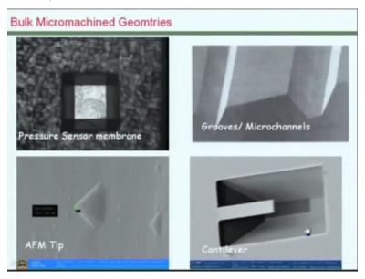
Bulk micro machining also discussed can be used for various devices as you see here one can built cavities one can built tip like structures, one can build cantilevers or gross using bulk micro machining process, all those processes have been discussed separately.
