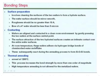
So as I mentioned preparing the surface and retaining the roughness and bow of the wafer within control is the key thing in the success of bonded wafers by this approach. After that just like you put 2 glass pieces together here you know we need to make them in contact and apply the temperature and then make them to bond together and usually we anneal it higher temperatures so that permanent contact is made.
