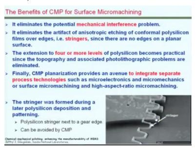
So there is also another advantage in using CMP especially for surface micro-machining. It is the removal of what is known as stringers. When there is this continuous processes you know, because this deposition is conformal, the layer would go down and add to the sides and essentially it may remain even after etching and a thin string kind of thing could remain and that is known as the stringer.
