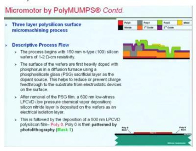
This approach essentially has 3 layers of polysilicon by surface micro-machining such complicated looking geometries could be fabricated. The detailed process flow available from the website has been discussed here. We start with a regular silicon wafer and build all these
