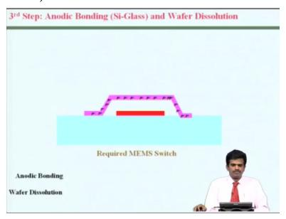
The next is essentially the anodic bonding which could be used to bond silicon and glass wafers. So these are added together bonded together and then we essentially dissolve this gray shaded region of silicon and after that what would remain is this structure that you see there. So in this
