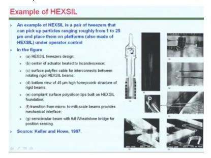
Fairly long and thick, vertically thick kind of geometries could be built by this approach. Obviously from the Mesoscale or large-scale geometries that you see when you would need such long beams you need to provide sufficient mechanical support and which is essentially provided by those honeycomb structure. So these could be fabricated by the geometries such as this could be fabricated by the process steps that are developed well over decade ago.
