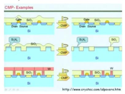
The use of CMP is very clear from the pictures that you see here. As you could see when you have the electrodes built on silicon and then we add the oxide layer above it, the oxide layer will have this bounce, it could be removed or you can even remove you know layer almost entirely by
