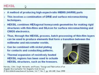
The next approach again fairly established for building a high aspect ratio microstructures is known by the acronym HEXSIL which has this hexagonal honeycomb like geometries on silicon or polysilicon which could be, you know, the process steps are somewhat similar to micromachining and it is compatible with CMOS based electronic processes. So this is a truly batch processing based approach.
