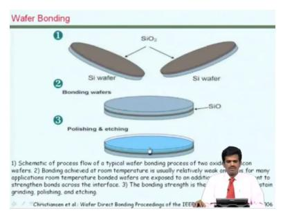
So how do we add wafer on to the surface of a partially made structure? To do that there are various approaches of attaching 2 wafers. May be silicon to silicon, maybe silicon to glass, various options are available to do that and basically what we do is that we start with these 2 wafers in the silicon to silicon case, we have an outside layer in between which essentially facilitates this close bonding between them.
