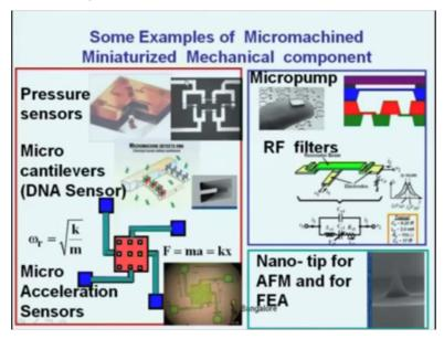
Now some examples of micromachined miniaturized mechanical components. I am just showing this in one slide to give a glimpse of some of these devices. For example, here, you have just a 3 dimensional schematic of a pressure sensor and here you have a photograph of the pressure sensor chip part of that shown here. The white what you see is the aluminium interconnection and there are 4 resistor located here 1, 2, 3, 4.
