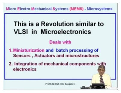
Now these microsystems or microelectromechanical systems is actually a revolution, which is similar to the VLSI in microelectronics and as you know that the VLSI began with a single transistor in 1947 when it was invented by Bardeen, Brattain and Shockley who won the noble prize for transistors. At the time, it was in large size single devices. Later on, the miniaturization of those devices was possible and that was possible in a big way.
