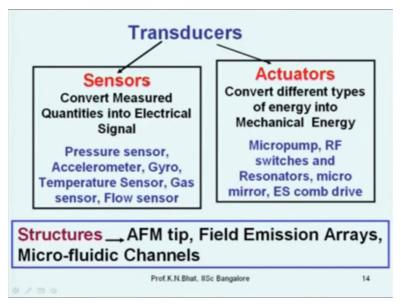
Now once again, I am touching upon this topic. Generally, you can classify it as sensors, actuators and structures, the MEMS and as I already pointed out sensors convert measured quantities into electrical signal to reiterate pressure sensors, accelerometers, gyro, temperature sensor, gas sensor, flow sensor all these come under this category and possibility of making them in micron size at least some dimensions in microns.
