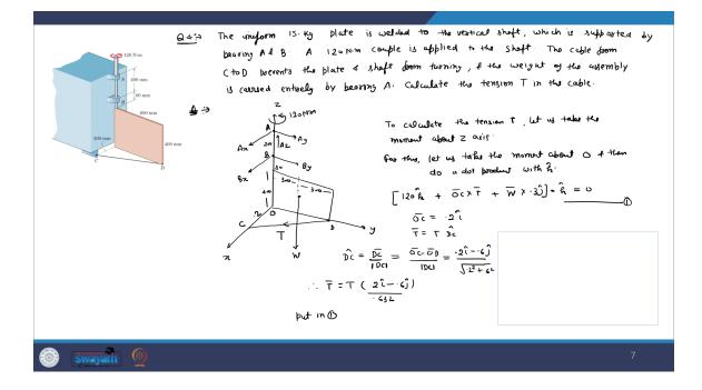
The uniform 15 kg plate is welded to the vertical shaft which is supported by bearing A and B, a 120 N.m. couple is applied to the shaft. The cable from C to D prevents the plate and shaft from turning and the weight of the assembly is carried entirely by bearing A and in the question it is asked you to calculate the tension T in the cable. So, first let us look at the free body diagram of this problem. So, first let me put the axis
