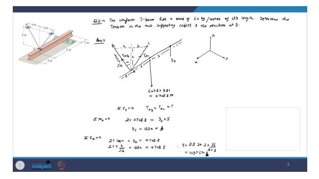
So, the problem statement is again following. Question number 2, the uniform *I*-beam has a mass of 60 kg/meter of its length and it is asked you to determine the tension in the two supporting cables and the reaction at D. So, first let us make the free body diagram of this problem. So, we have this *I*-beam and at a distance of 2 meter, we have two cables and in these cables because of the symmetry, the tension will be the same.
