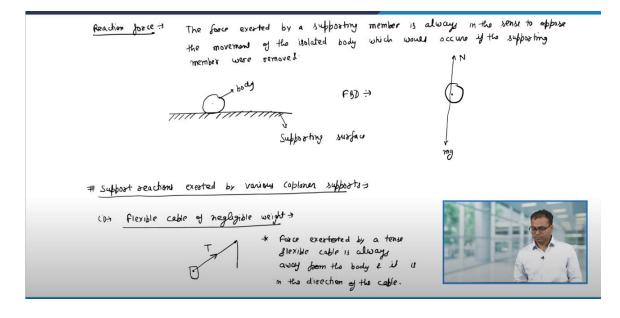
So, with this let me briefly discuss what are the reaction forces and what is the definition of that. So, the force exerted by a supporting member is always in the sense to oppose the movement of the isolated body which would occur if the supporting members were removed. There is nothing but the Newton's third law only. So, let us look at by an example. Suppose, I have a supporting surface and on top of it, I have a body.
