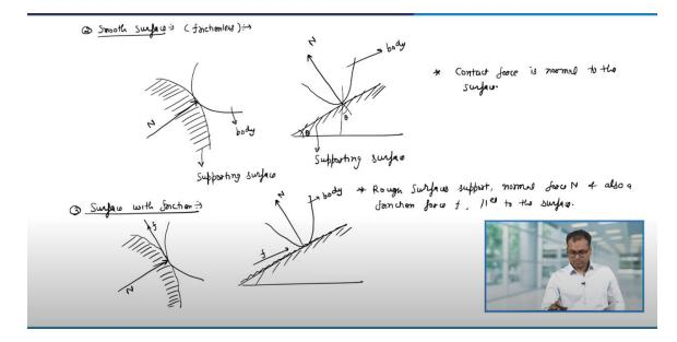
Now, let us say we have a smooth surface and this surface is smooth means it is frictionless. So, let us say I have a surface. So, this is my supporting surface and I have a body. In this case, the force will act normal to the surface. So, the support reaction will be like that.
