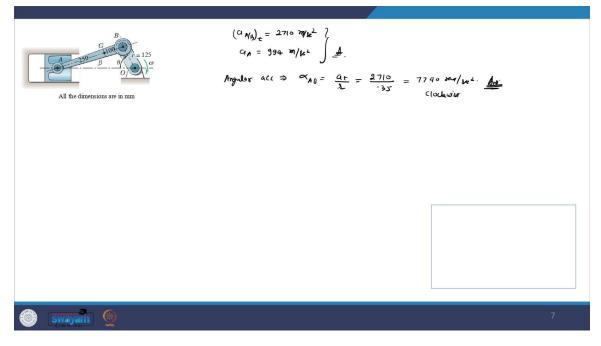
From here, we can find out that  $(a_{A/B})_t = 2710 \text{ } m/\text{sec}^2$  and  $a_A = 994 \text{ } m/\text{sec}^2$ . And the angular acceleration of *AB*, which is  $\alpha_{AB} = \frac{a_t}{r} = \frac{2710}{0.35} = 7790 \text{ } rad/\text{sec}^2$  in the clockwise direction.
